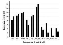
Figure 7 - Effect of ions and EDTA on enzyme activity.
