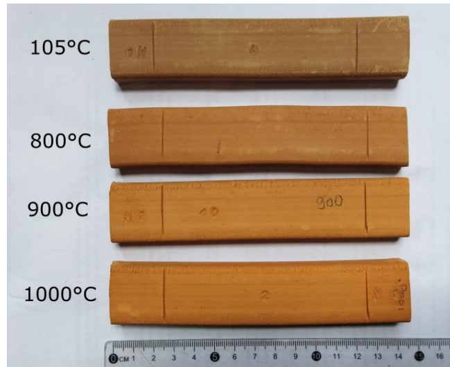
Figure 9 – Color of the specimens after firing.
