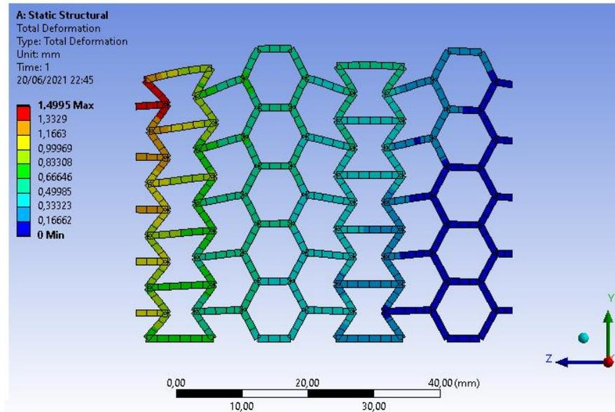
**Figure 14 – Front view of total deformation profile of each element in beam element simulation when applying a horizontal compression displacement of 1mm.**
