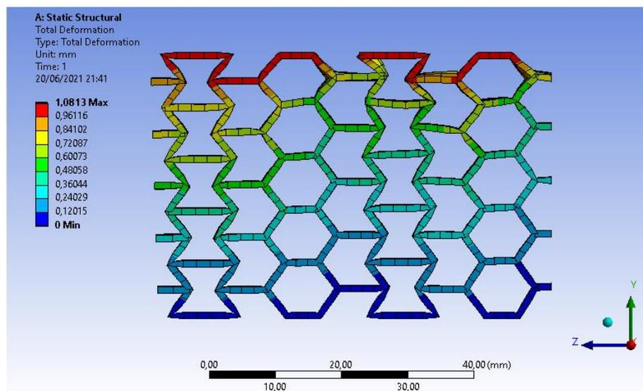
**Figure 12 – Front view of total deformation profile of each element in shell element simulation when applying a vertical compression displacement of 1mm.**
