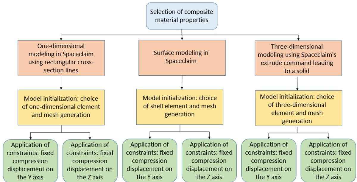
**Figure 2 – Flowchart showing simulation steps.**
