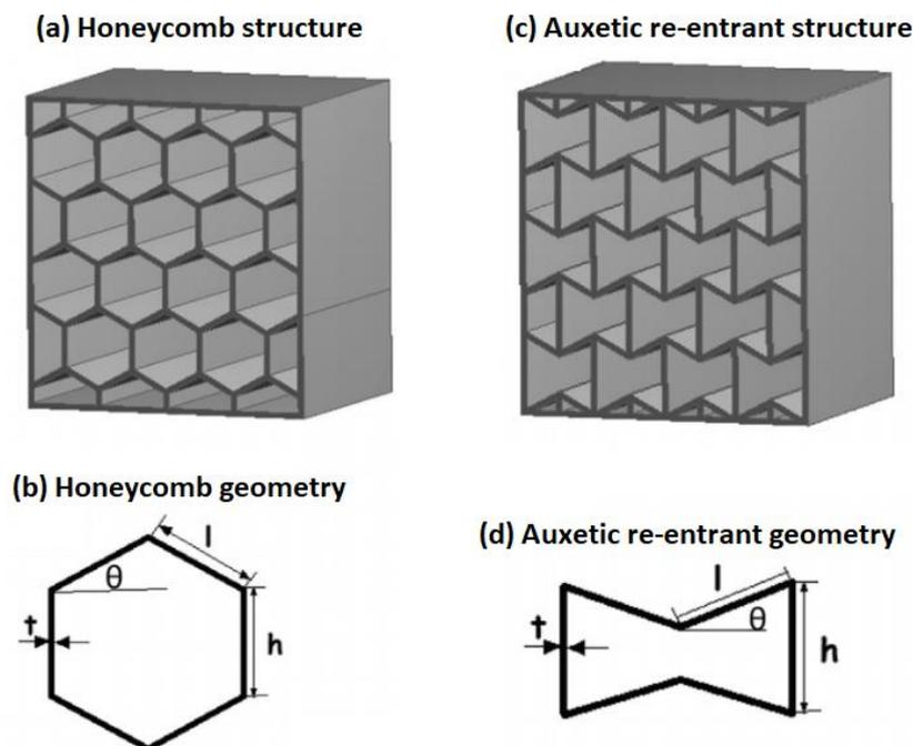
**Figure 1 – Honeycomb and re-entrant auxetic structures and geometries. (Adapted from Shruti *et al.*, 2021)**
