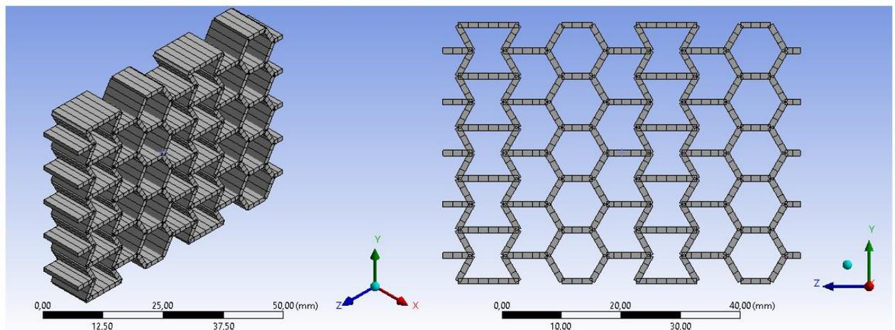
**Figure 6 – Frontal and isometric views of model meshing used for simulation of one-dimensional elements (beam).**
