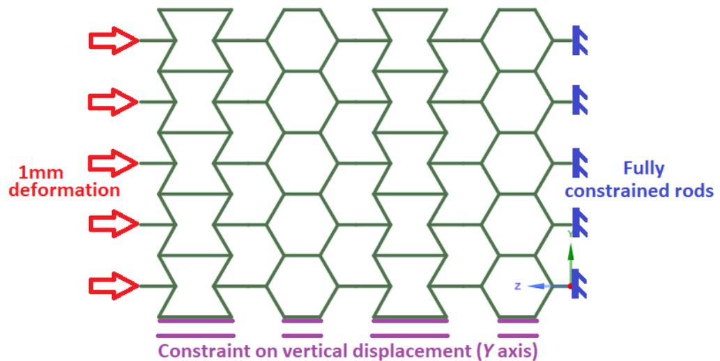
Figure 10 – Constraints of the second situation used for finite element simulations of beam, shell and body models (1mm compression displacement along Z-axis).
