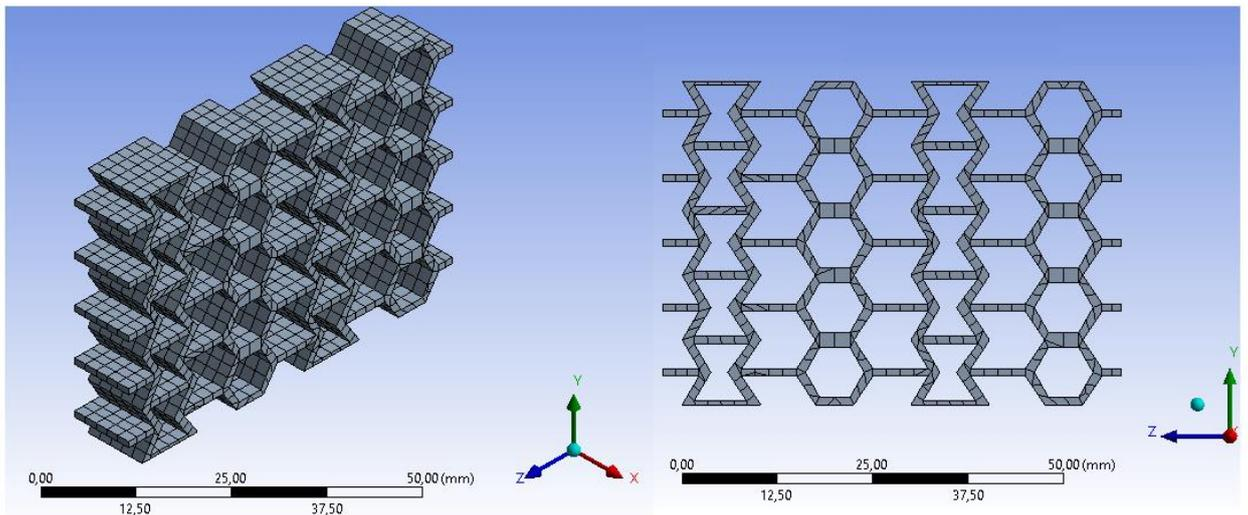
**Figure 8 – Frontal and isometric views of model meshing used for simulation of three-dimensional elements (solid body).**
