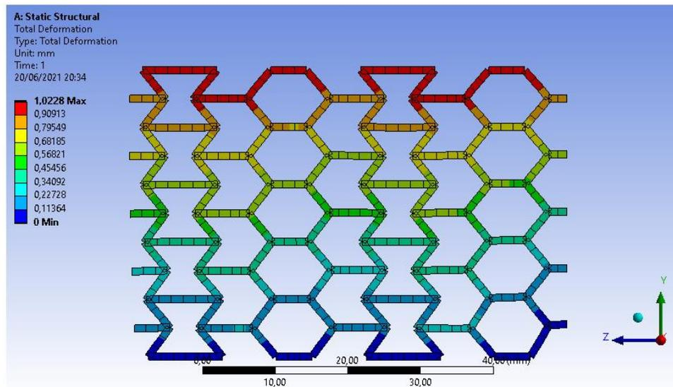
**Figure 11 – Front view of total deformation profile of each element in beam element simulation when applying a vertical compression displacement of 1mm.**
