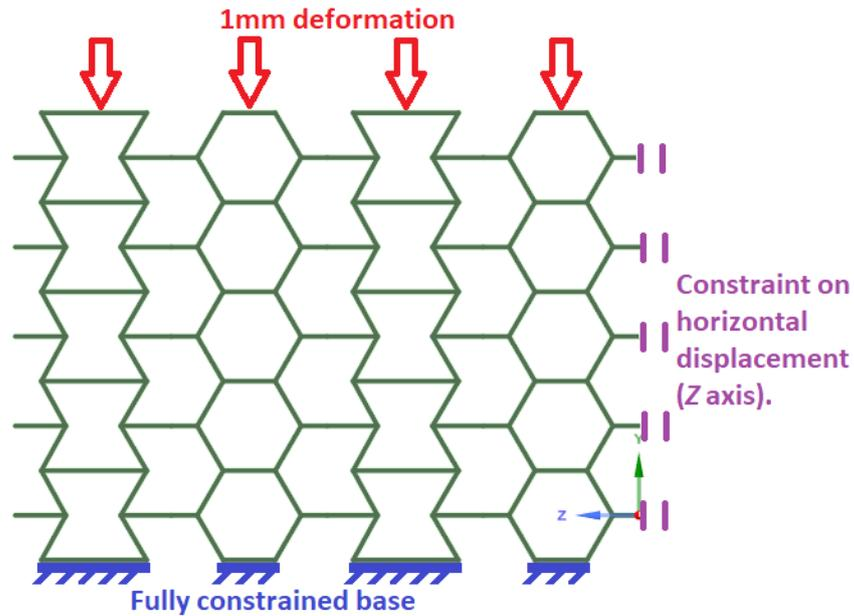
Figure 9 – Constraints of the first situation used for finite element simulations of beam, shell and body models (1mm compression displacement along Y-axis).
