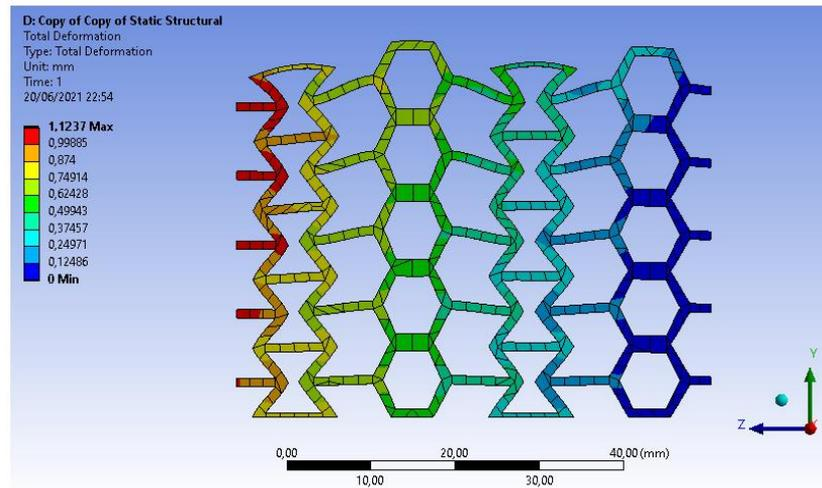
**Figure 16 – Front view of total deformation profile of each element in body element simulation when applying a horizontal compression displacement of 1mm.**
