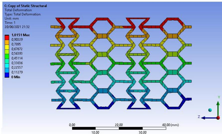
**Figure 13 – Front view of total deformation profile of each element in body element simulation when applying a vertical compression displacement of 1mm.**
