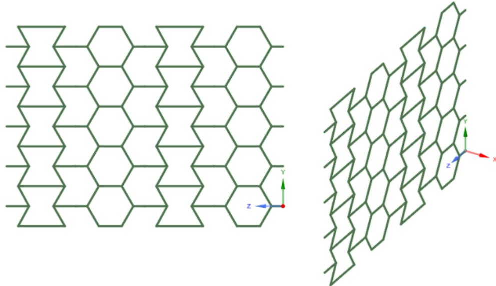
**Figure 3 – Frontal and isometric views of geometry generated in *Spaceclaim* used to perform simulations of one-dimensional elements.**
