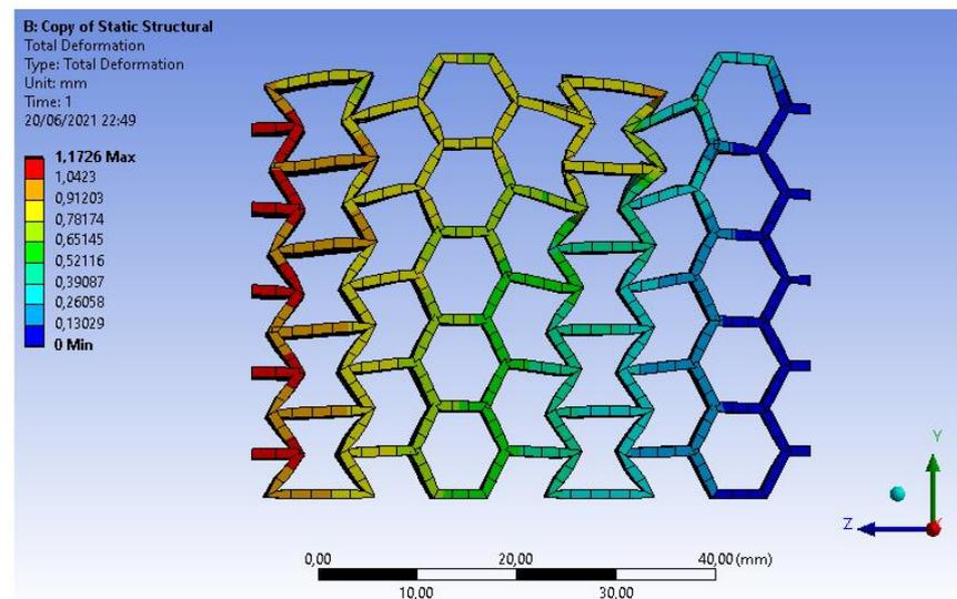
**Figure 15 – Front view of total deformation profile of each element in shell element simulation when applying a horizontal compression displacement of 1mm.**
