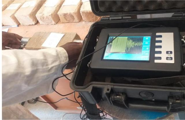
**Figure 8 - A device that measures the speed of sound.**
