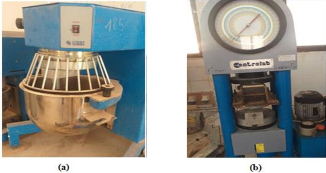
Figure 5 - Used laboratory equipment (a) Electric mixer (b) Hydraulic press
