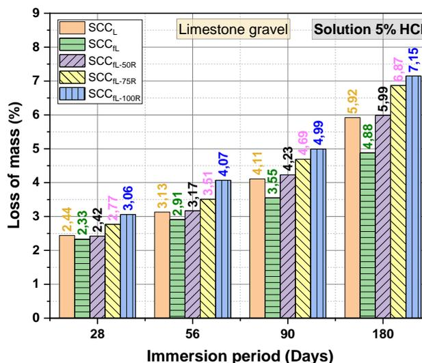
Figure 9 – Variation in the mass of SCC according to the age of immersion in HCl
