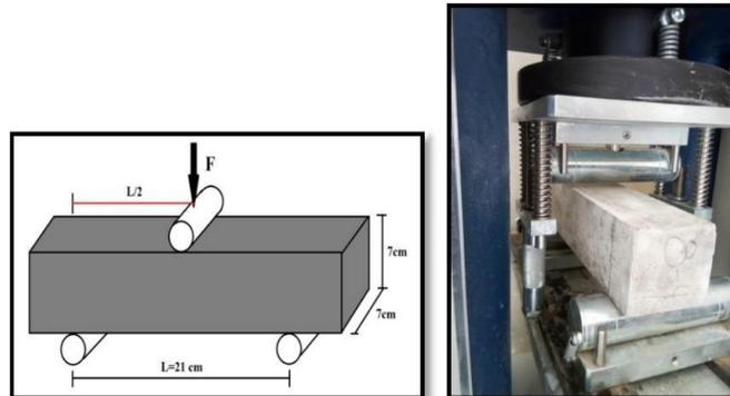
**Fig. 6 – Device and static diagram for the bending tensile test.**
