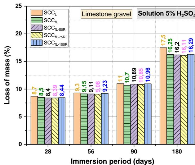
Figure 10 – Variation in SCC mass as a function of H<sub>2</sub>SO<sub>4</sub> immersion age.
