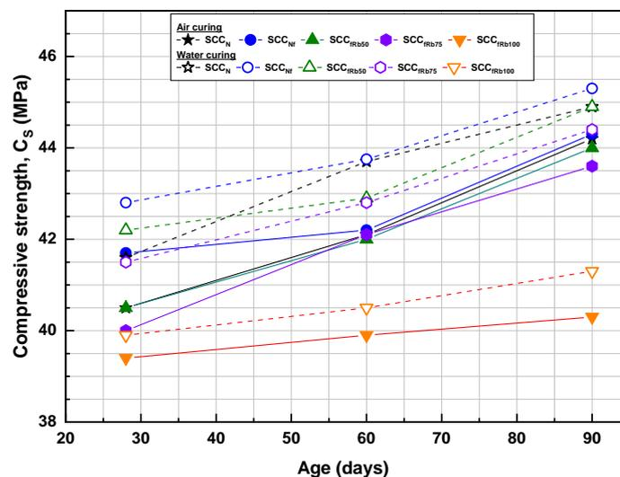
Fig. 5 – Evolution of the compressive strength  $C_s$  of the concretes according to their age.
