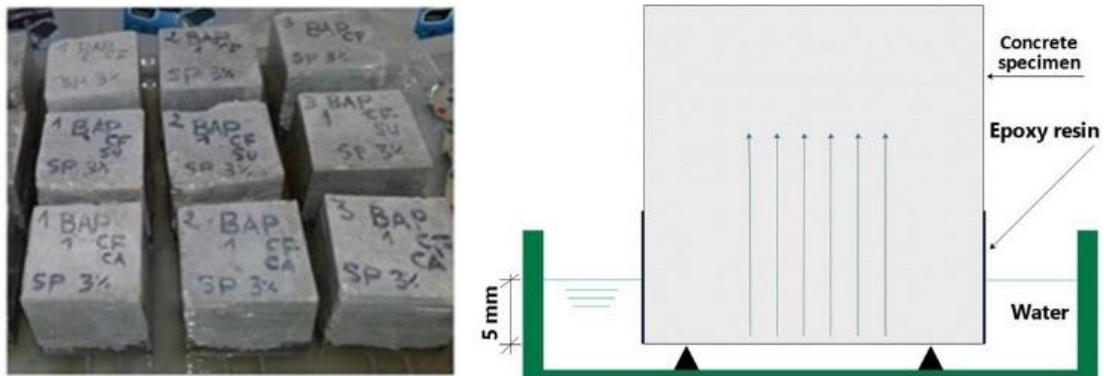
**Figure 2 – Test of the absorption of water by capillaries.**
