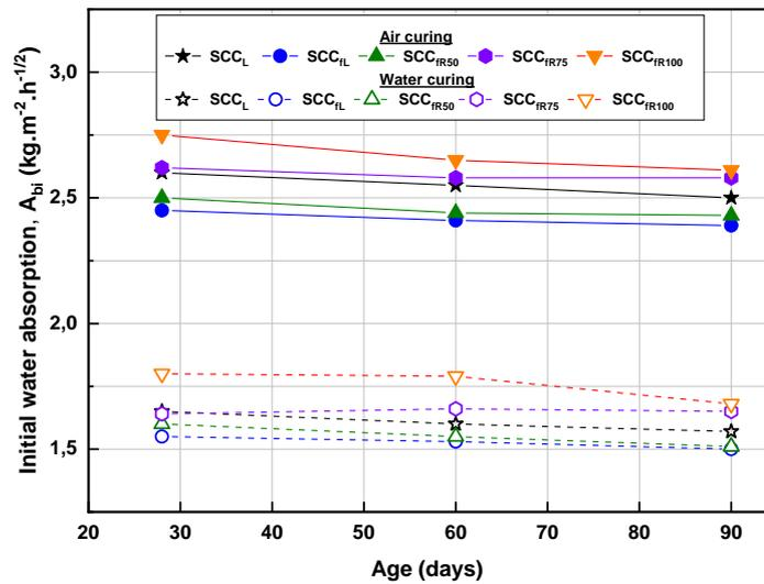
Figure 3 – Absorption of initial water (A<sub>bi</sub>) of the all.
