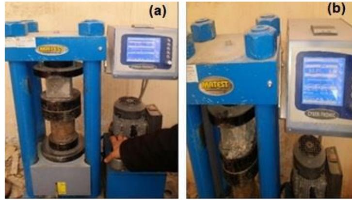
Fig. 4 – Test-tubes before and after crushing.
