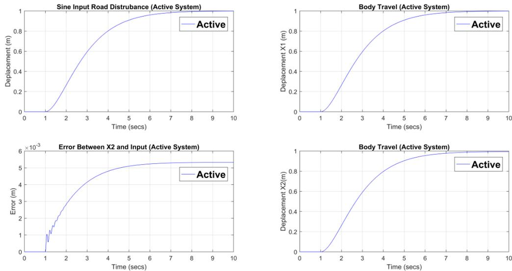
**Figure 4 - Response of the active suspension to a graded unit step input**
