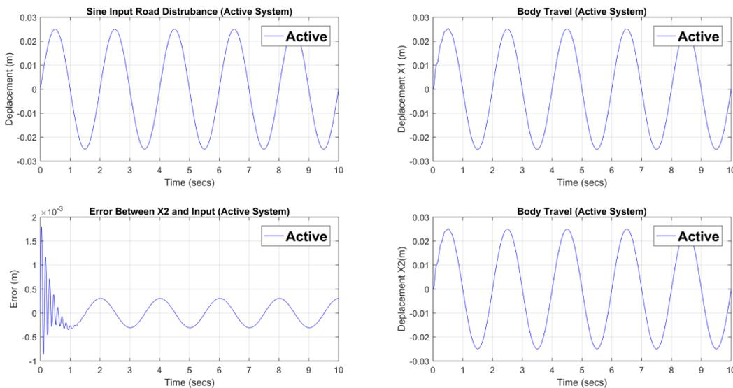
**Figure 3 - Response of the active suspension to a sinusoidal input**
