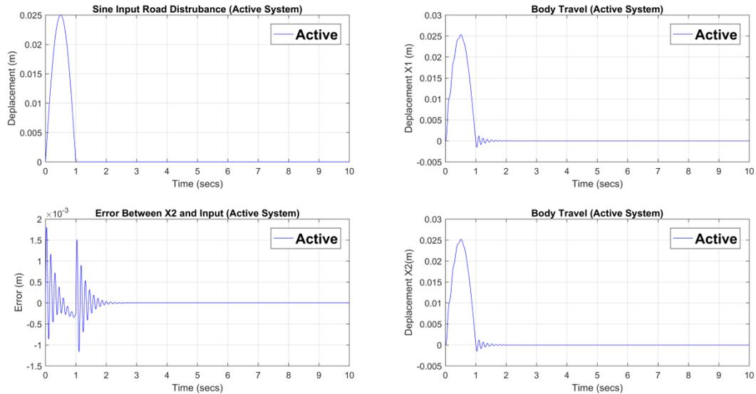
**Figure 2 - Response of the active suspension to a sudden road input**
