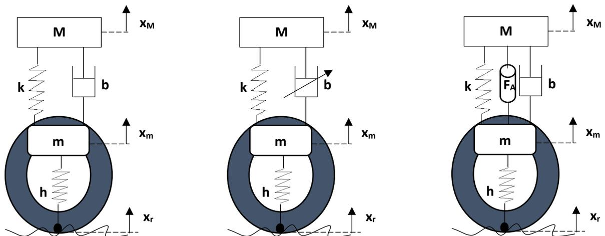
Figure 1 – Quarter Vehicle Suspension (a) Passive (b) Semi-Active (c) Active
