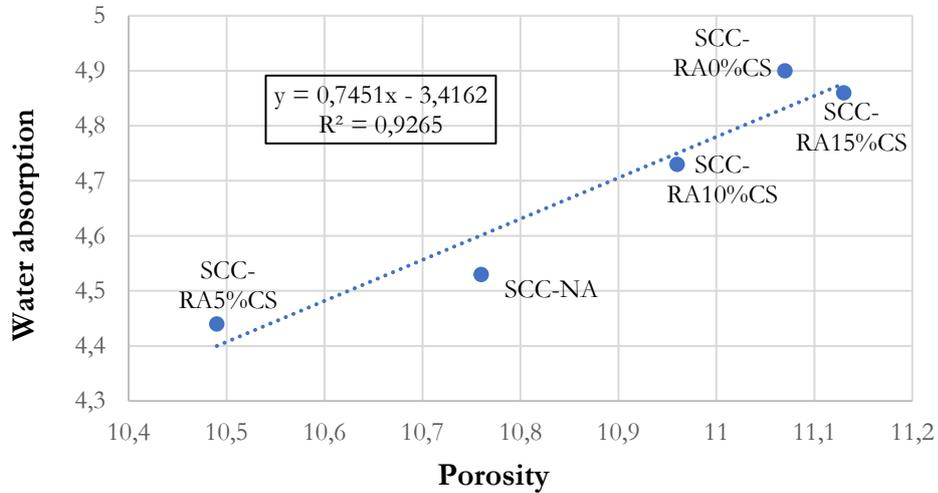
Figure 12– Relationship between the water absorption and porosity.
