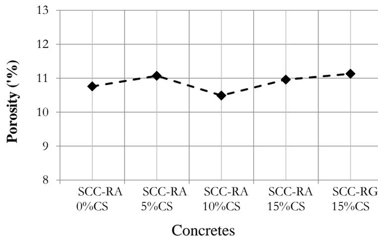
**Figure 9– Effect of CS on porosity of SCC.**
