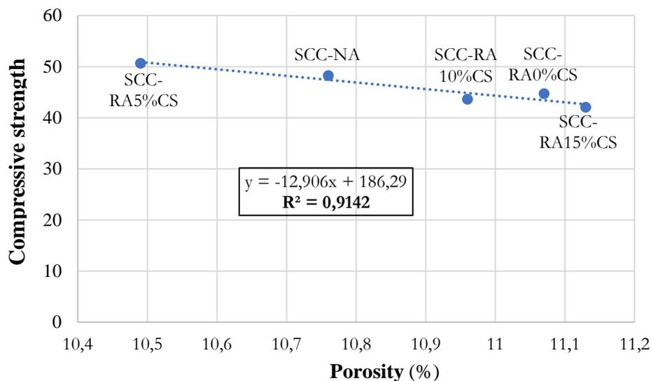
Figure 11– Relationship between the compressive strength and porosity.
