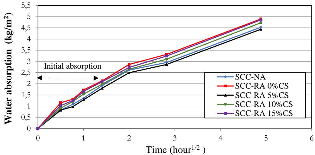
Figure 10– Evolution of SCC capillary absorption according to CS.
