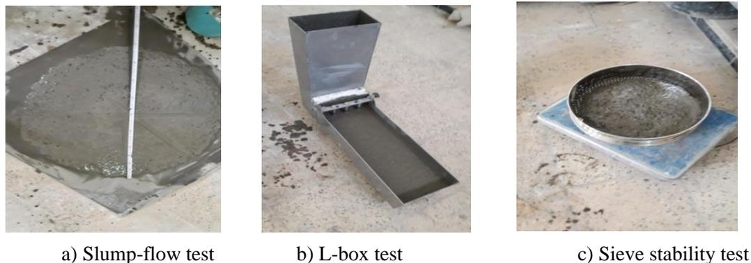
**Figure 6– Workability tests.**
