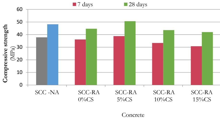
**Figure 8– Effect of CS on compressive strength of SCC.**
