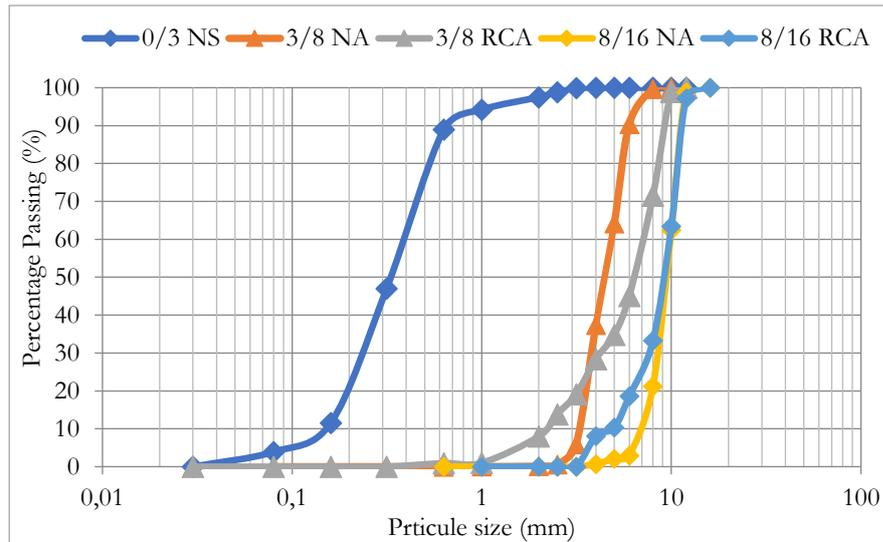
**Figure 4– Particle size distributions of aggregate used.**
