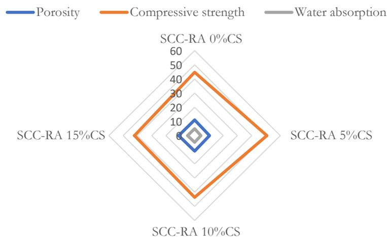
Figure 13– Effect of CS on physical and mechanical proprieties of SCC.
