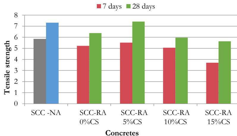
**Figure 7– Effect of CS on tensile strength of SCC.**
