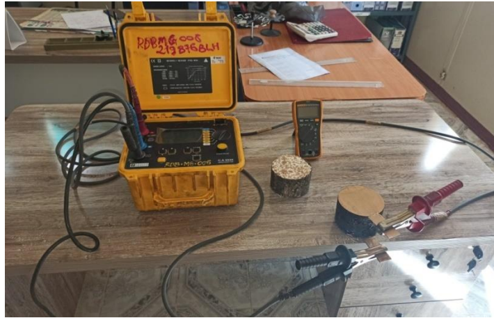
Figure 6 – Measures electrical resistance using the two-point method.
