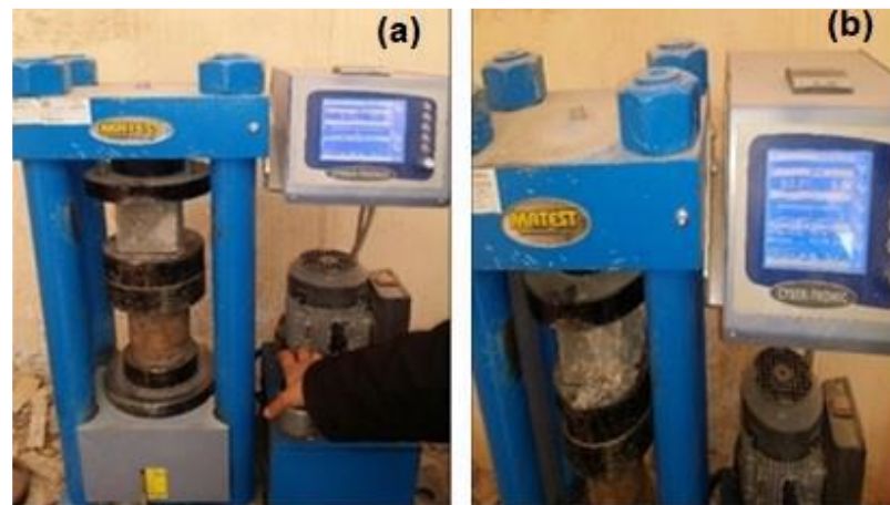
Figure 2 – (a) Specimens before crushing, (b) Specimen after crushing (breaking).
