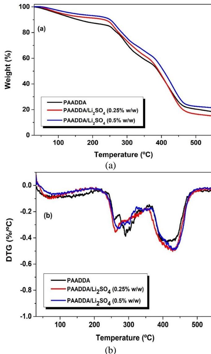
**Figure 2.** (a) TGA and (b) DTG curves for pristine PAADDA and PAADDA/Li<sub>2</sub>SO<sub>4</sub> films.
