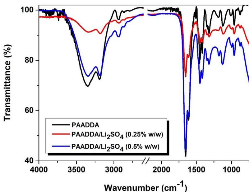
**Figure 1.** ATR-FTIR spectra of pristine PADD A and PAADDA/Li<sub>2</sub>SO<sub>4</sub> films.
