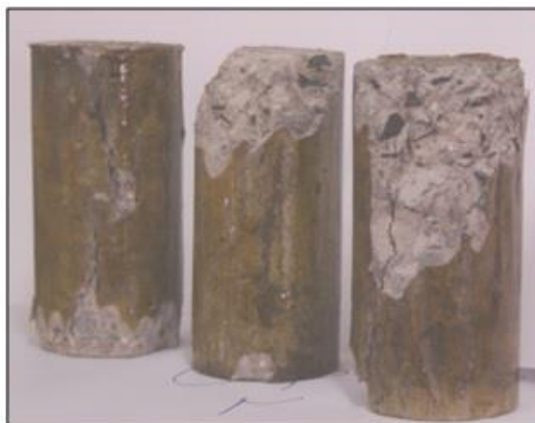
Figure 12 – After crushing, concrete specimens without reinforcement.
