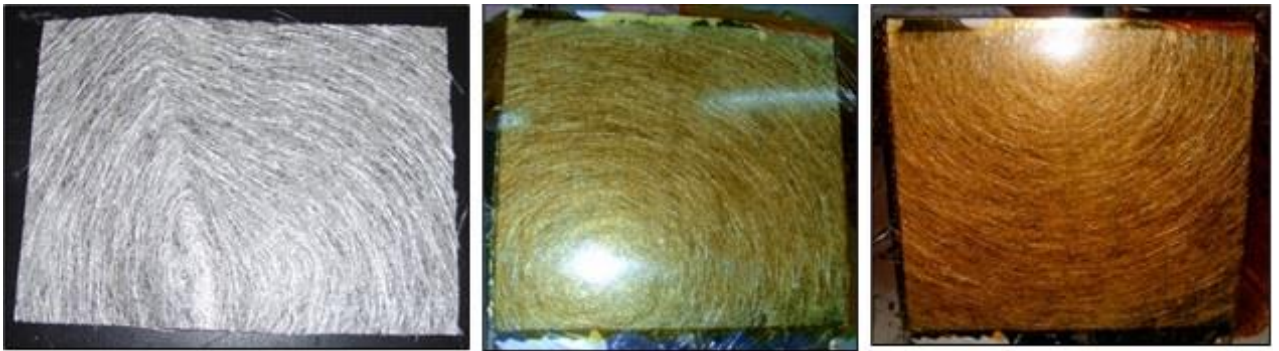
Figure 5 – Fiberglass cutting and plates of composite material (fiberglass + resin) after hardening.
