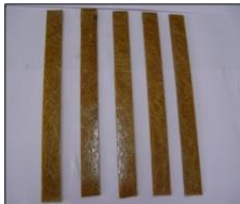
Figure 6 – Cutting of composite material specimens.
