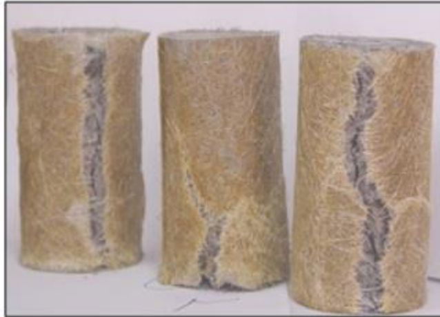
Figure 16 – Failure conditions of concrete specimens confined by 1-ply GRP.
