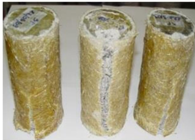
Figure 18 – Failure conditions of concrete specimens confined by 3-ply GRP.
