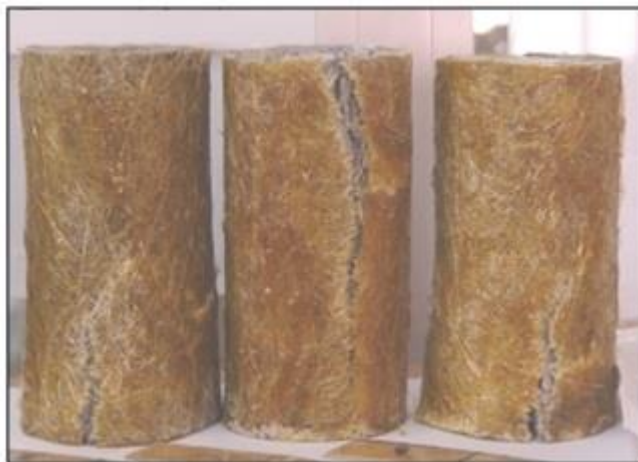
Figure 17 – Failure conditions of concrete specimens confined by 2-ply GRP.
