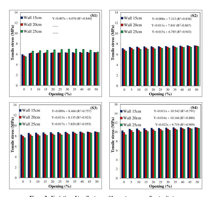
Figure 2 - Variation of tensile stress with apertures according to site type.
