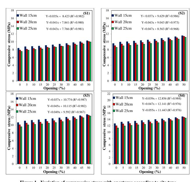
Figure 1 - Variation of compressive stress with apertures according to site type
