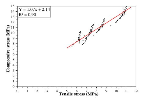
Figure 3- Correlation between compressive and tensile stresses.
