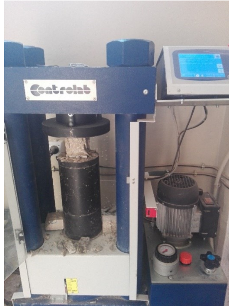
Figure 3 – Concrete axial compression test equipment.
