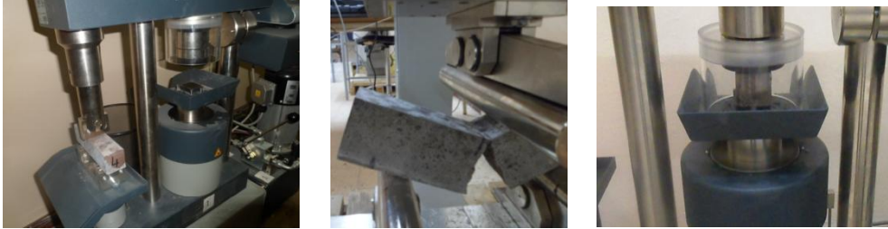
Figure 6 – Essai de flexion & Essai de compression
