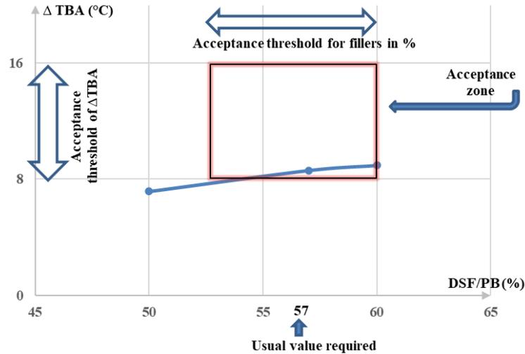
Figure 9 - Variation in  $\Delta TBA$  as a function of the ratio of DSF to PB.
