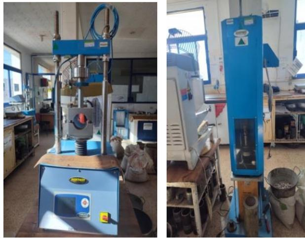
Figure 8 - The equipment for the MARSHALL test.
