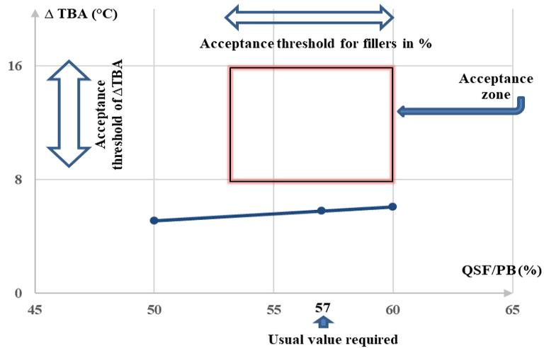
Figure 10 - Variation in  $\Delta TBA$  as a function of the ratio of QSF to PB.
