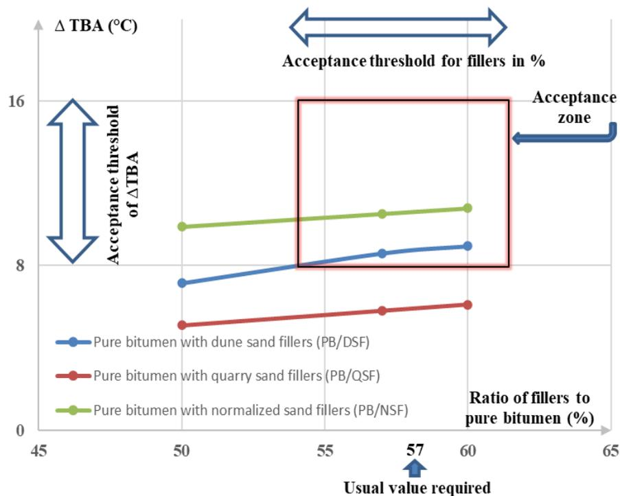
Figure 12 - Variation in  $\Delta TBA$  as a function of the proportion of DSF, QSF and NSF to PB.
