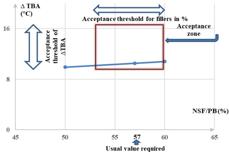
Figure 11 - Variation in  $\Delta TBA$  as a function of NSF to PB ratio.
