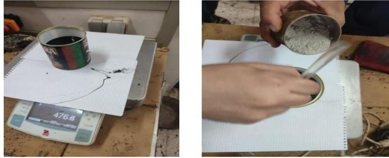
Figure 4 - Preparation of bitumen/filler
