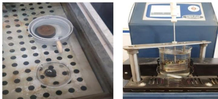
Figure 6 - Testing the softening point of the PB+DSF mixture.
