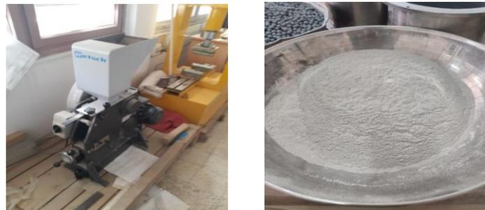
Figure 2 - Dune sand fillers DSF after milling
