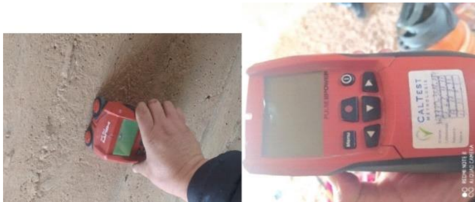
Figure 8 - Multi-detector wall scanner. Source: Authors (2023).
