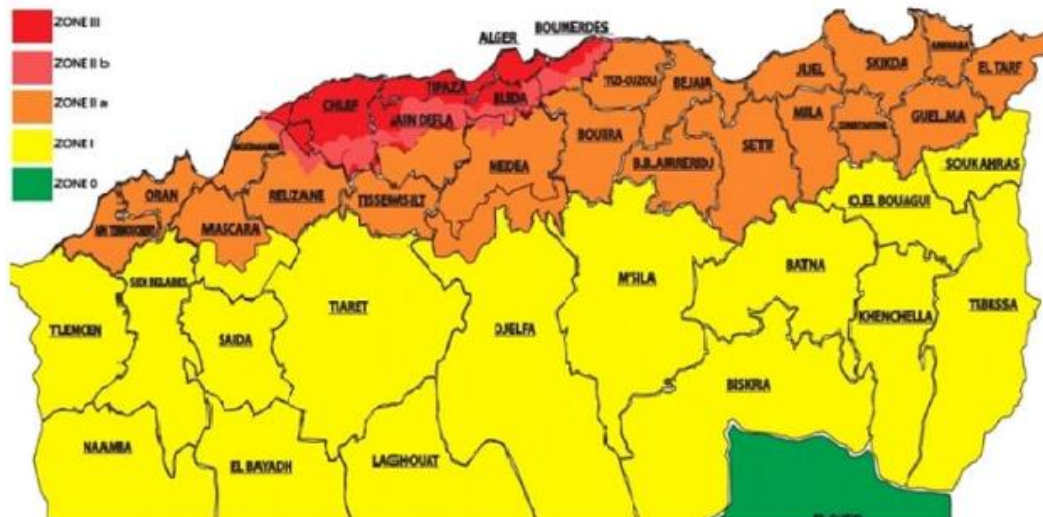
Figure 2 - Seismic zoning map of Algeria according to RPOA 2008. Source: (RPOA, 2008)
