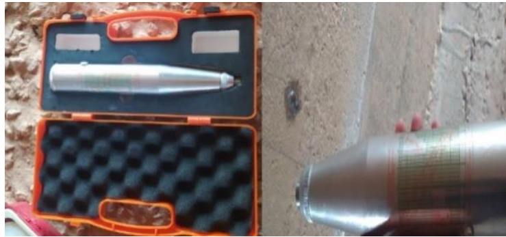
Figure 10 - Concrete strength measurement apparatus (concrete sclerometer). Source: Authors (2023).
