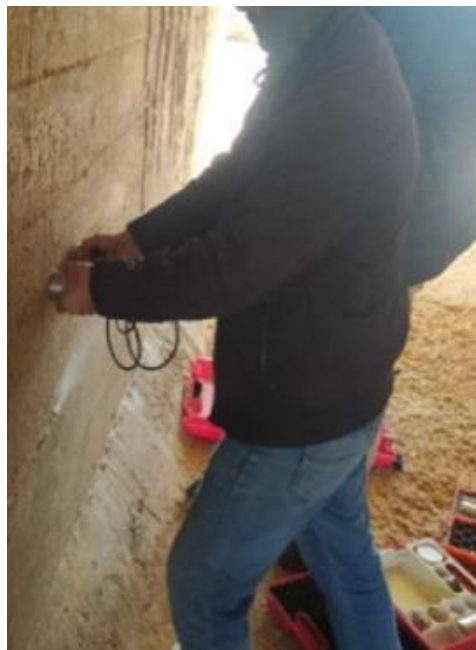
Figure 9 - Measurement of propagation speed (TICO-type ultrasound). Source: Authors (2023).
