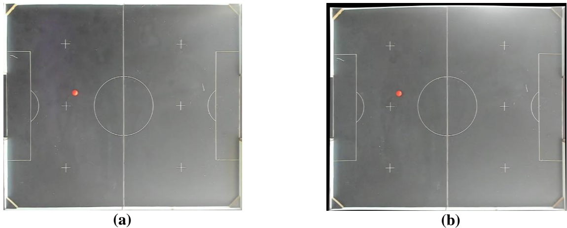
Figure 14 - Top view of the soccer field after alignment (a) and calibration of the camera's optical distortion (b).
