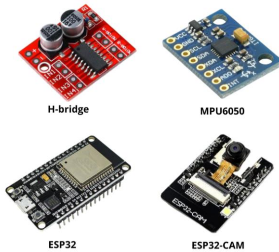
Figure 5 – The components used in the project: H-bridge, MPU6050, ESP32 and ESP32CAM.
