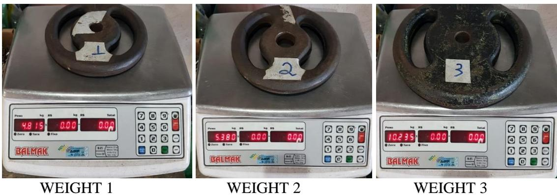
Figure 8 - Standard weights used in calibration (4,815kg, 5,380kg, 10,235kg respectively). Source: Authors (2024).
