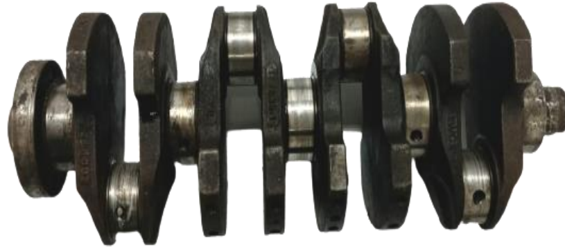
Figure 1 – This is a crankshaft of the four-stroke engine used as a specimen in the balancing rig.
