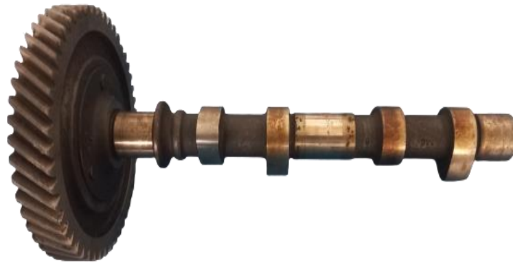
Figure 2 – This is a camshaft of an engine used as a specimen in the balancing rig.
