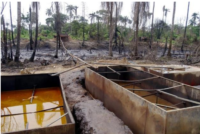
Figure 7. Zinc reservoir for storage of raw crude (Source: Adunbi, 2022).
