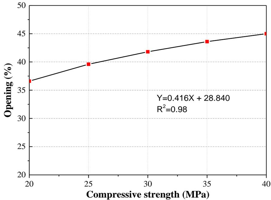
**Figure 7.** Optimization of openings in shear walls based on compressive strength.
