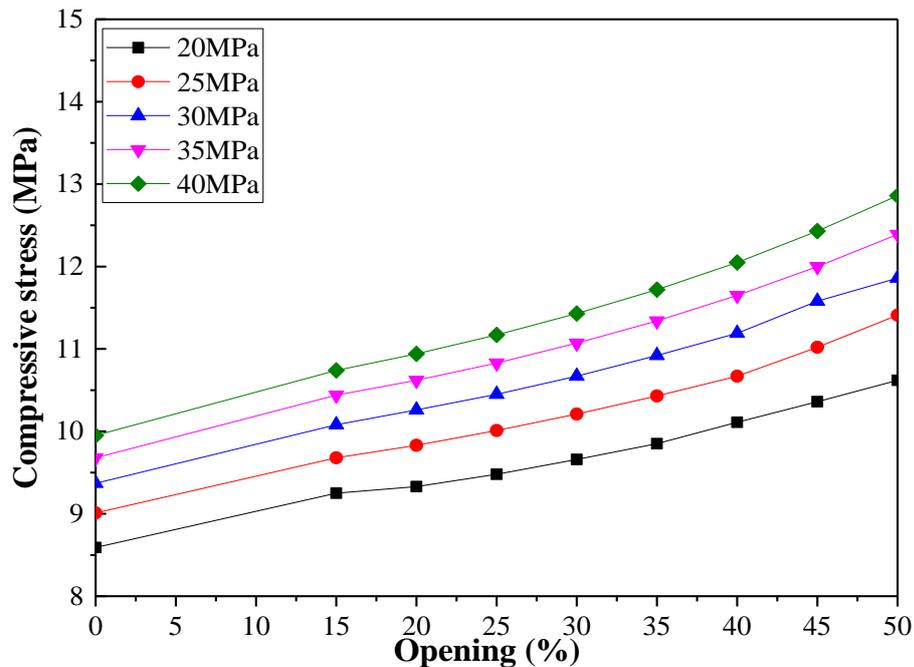
Figure 3. Compression stresses based on openings in shear walls.
