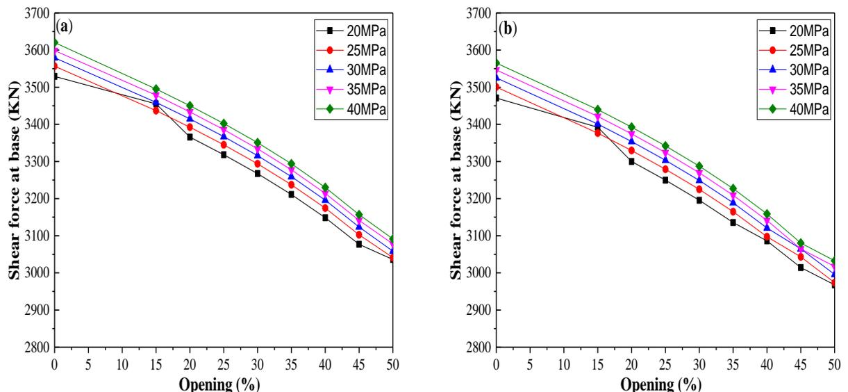
**Figure 1.** Evolution of shear forces in buildings based on openings in shear walls: (a) X-Direction, (b) Y-Direction.
