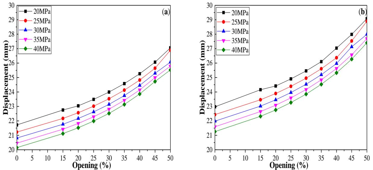
**Figure 2.** Evolution of total displacements in buildings based on openings in shear walls: (a) X-Direction, (b) Y-Direction.
