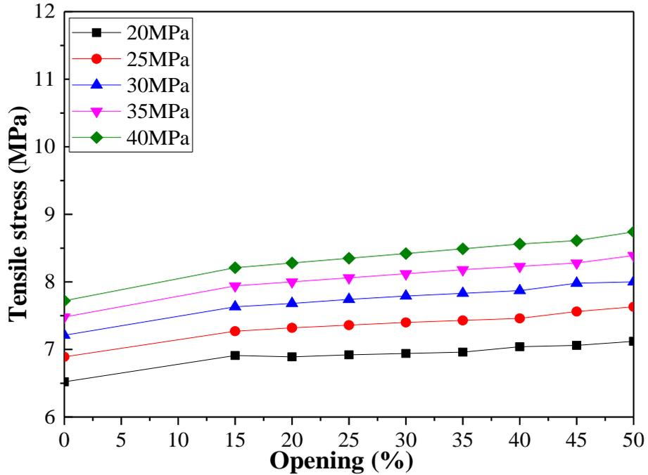
Figure 4. Tensile stresses based on openings in shear walls.
