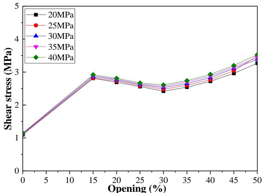
Figure 6. Shear stresses are based on openings in shear walls.
