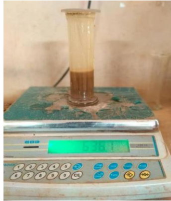
Figure 1: Measurement of Glass Jar Weight for Specific Gravity Assessment
