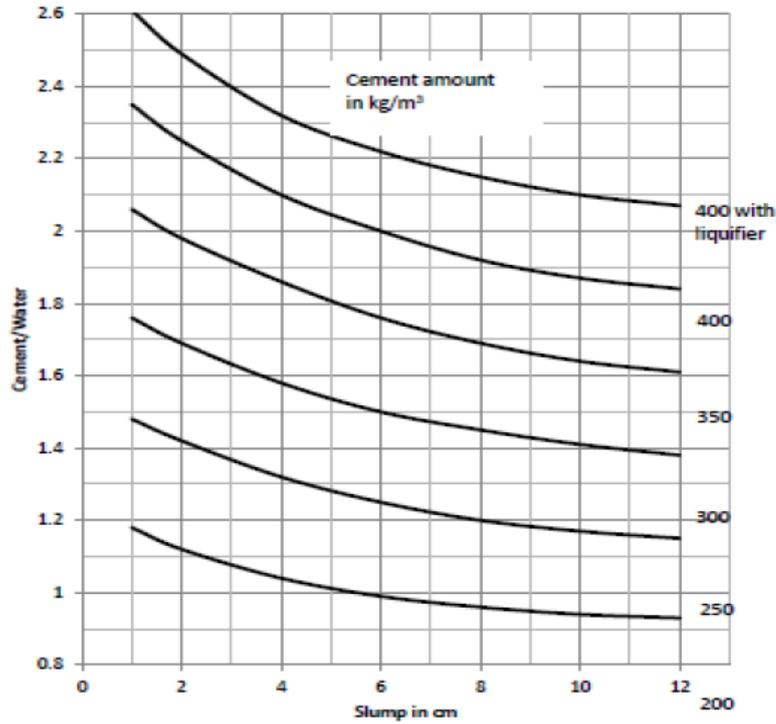
**Figure 1** - Estimation of the cement content to be used based on the water-to-cement ratio and workability (Dreux, G., 1981).
