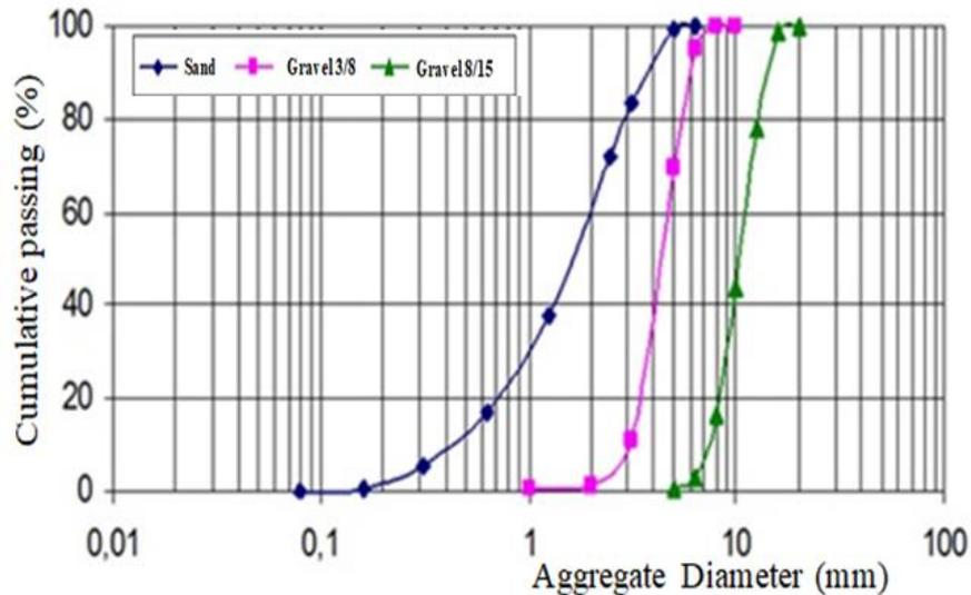
Figure 4 - Curves of granulometric analyses of aggregates.
