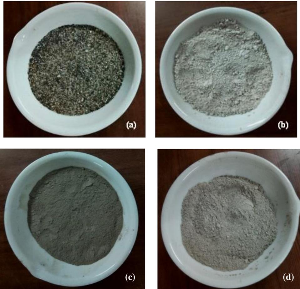
**Figure 3 - Materials employed in this investigation: (a) Clean sand, (b) clay, (c) silt, (d) Silt-clay mixtures.**
