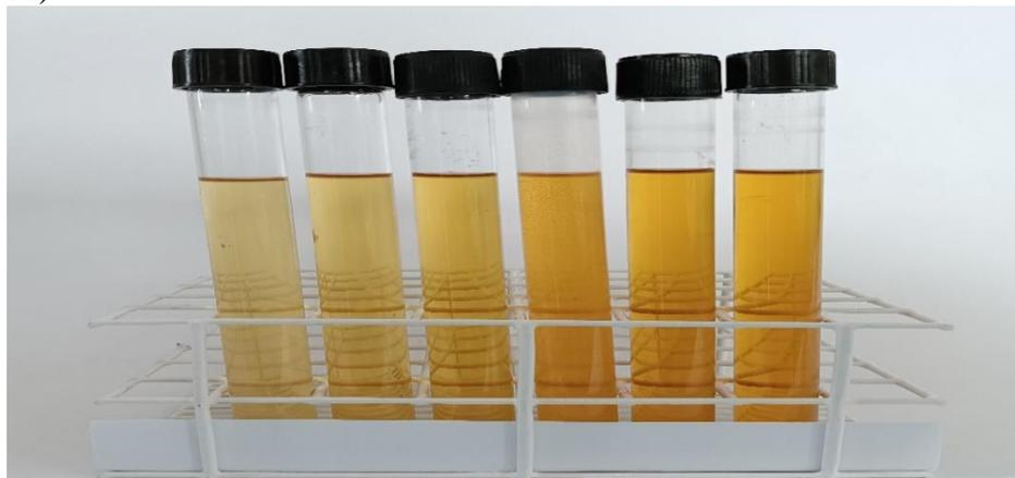
**Figure 14 – Coloring of NaOH solutions after processing with coconut fiber**
