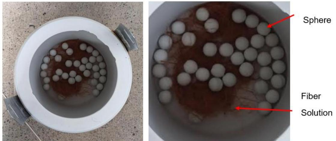
**Figure 2 - Mill jar at rest, with spheres, NaOH solution and coconut fibers**
