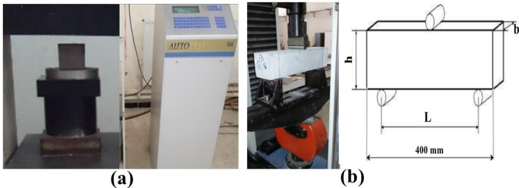
Figure - 4 Apparatus used for the compressive (a) and three-point flexural (b).
