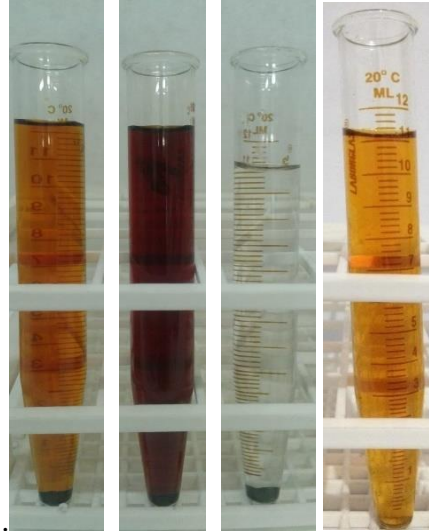
Figure 6 - Result of resolubilization with potassium iodide solution of molecular iodine containing adsorbed AM obtained by adsorptive tests with (a) fragmented commercial iodine, (b) commercial iodine spheres, (c) iodine recovered from the degradation oxidative process with hydrogen peroxide and (d) only commercial iodine without AM adsorbed.
