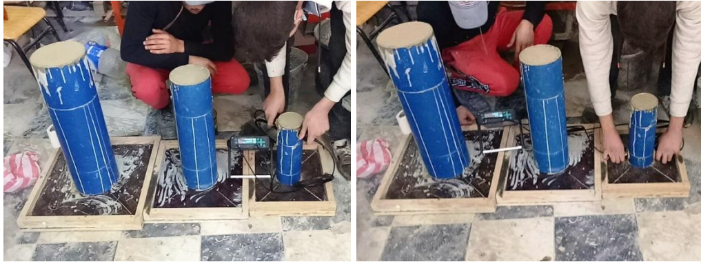
Figure 6 - Effect of sample size on concrete segregation index measured by ultrasonic pulse velocity (UPV).
