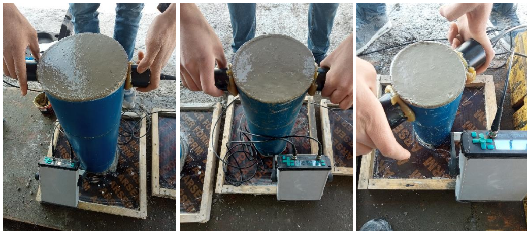
Figure 4 - Ultrasonic pulse velocity test for segregation assessment in a concrete column.
