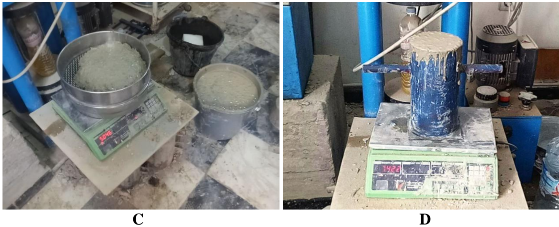
Figure 2 - (A) Abrams' cone flow test, (B) L-box test, (C) Sieve stability test and (D) Concrete density tests.
