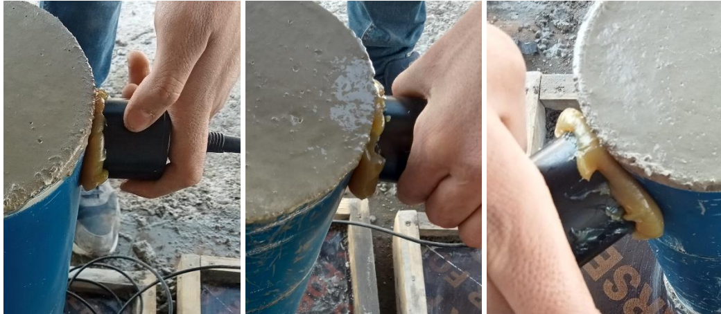
Figure 5 - Application of the ultrasonic pulse velocity (UPV) method to assess segregation (V1, V2 and V3).
