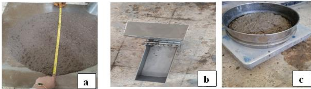
Figure 5 - Fresh state testes: (a) Slump flow test, (b) L-Box test, (c) Sieve stability test.
