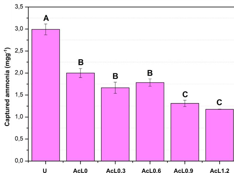
**Figure 8 - Amount of ammonia captured per the amount of N applied as uncoated urea (U), coated with 2% cellulose acetate (AcL0), and with the combination of 2% cellulose acetate with increasing lignin proportions: 0.3 % (AcL0.3), 0.6 % (AcL0.6), 0.9 % (AcL0.9), and 1.42 % (AcL1.4).**
