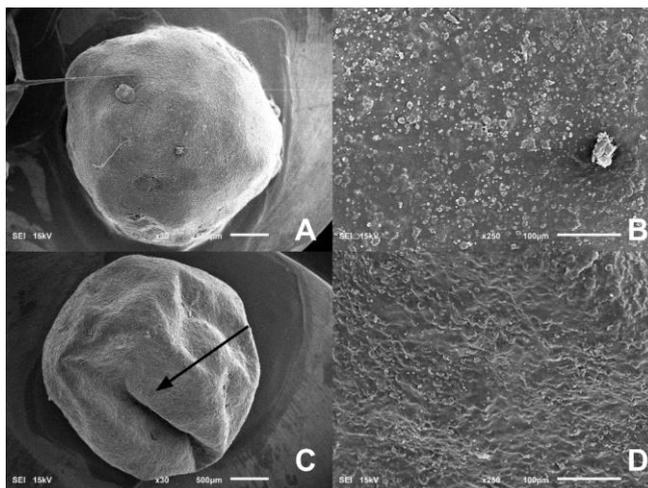
**Figure 9 - Scanning electron microscopy images of urea granule coated (A, 30x and B, 250x) and of the remaining coating film after urea solubilization (C and D). Coating formulation AcL0.3.**
