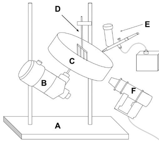
**Figure 1 - Plate (or disc) granulator used for coatings A: Bracket; B: mechanical agitator; C: rotating disc; D: radial shovel; E: Micro spray with compressor; and F: heat blower.**
