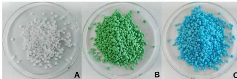
**Figure 3 - Uncoated urea granule (A) and coated with 2% cellulose acetate dyed in green (B) and blue (A), to demonstrate the uniformity of the coating.**
