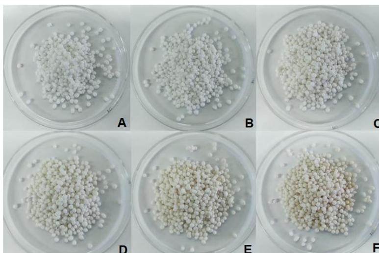
**Figure 5 - Uncoated urea granules (A), coated with (B) cellulose acetate, 2% (AcL0), and the combination of 2% cellulose acetate with increasing proportions of lignin 0.3% (AcL0.3) (C), 0.6% (AcL0.6) (D), 0.9% (AcL0.9) (E), and 1.2% (AcL1.2) (F).**
