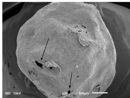
**Figure 7 - Image of urea granule coated with the formulation AcL0.9, evidencing discontinuity in the covering film (and holes).**
