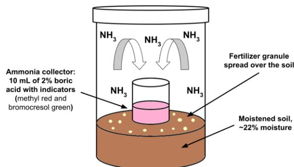
**Figure 2 - Static system to evaluate  $\text{NH}_3$  volatilization, consisting of the incubation chamber and the collection vessel.**
