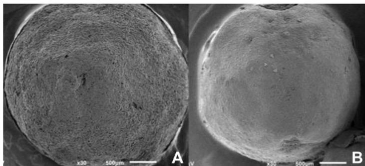
**Figure 4 - SEM images of urea granules without coating (A) and with coating (B)**
