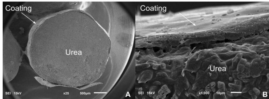
**Figure 6 - SEM images of the (A) cross-section of the urea granule coated with the formulation AcL0.6, and (B) detail of the interaction of the coating film with the granule surface.**
