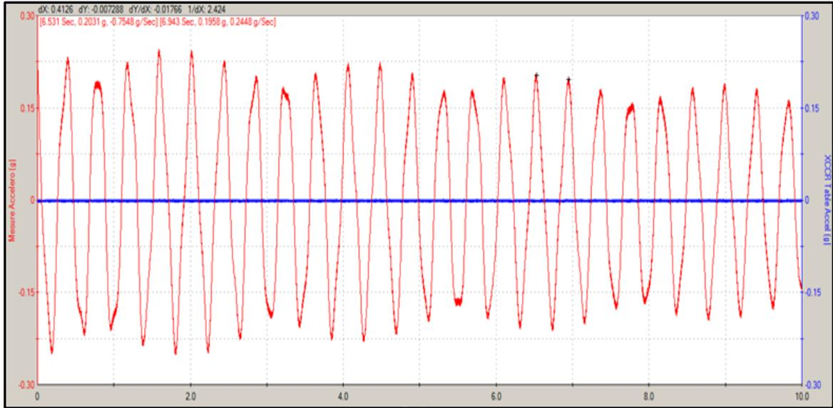
Figure 11 – Second free vibration test of the model
