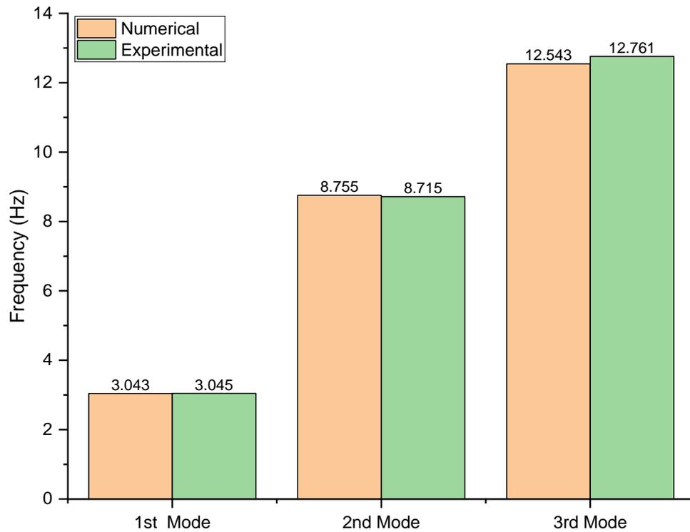
**Figure 13 – Comparison of numerical and experimental frequencies**
