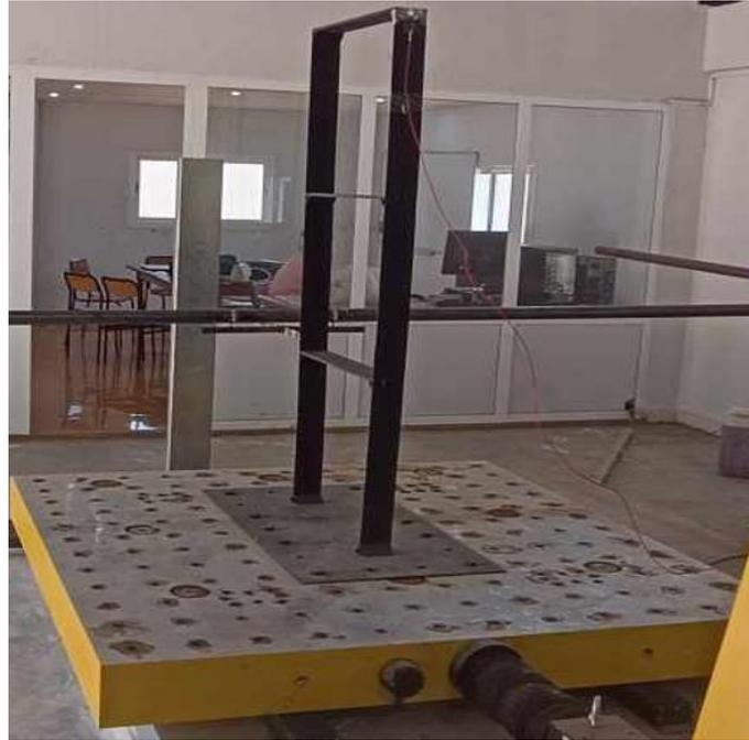
**Figure 2 – The 1:6 reduced-scale model fixed at the shaking table**
