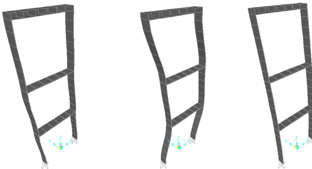
**Figure 8 – The three first vibration modes of the finite elements model**
