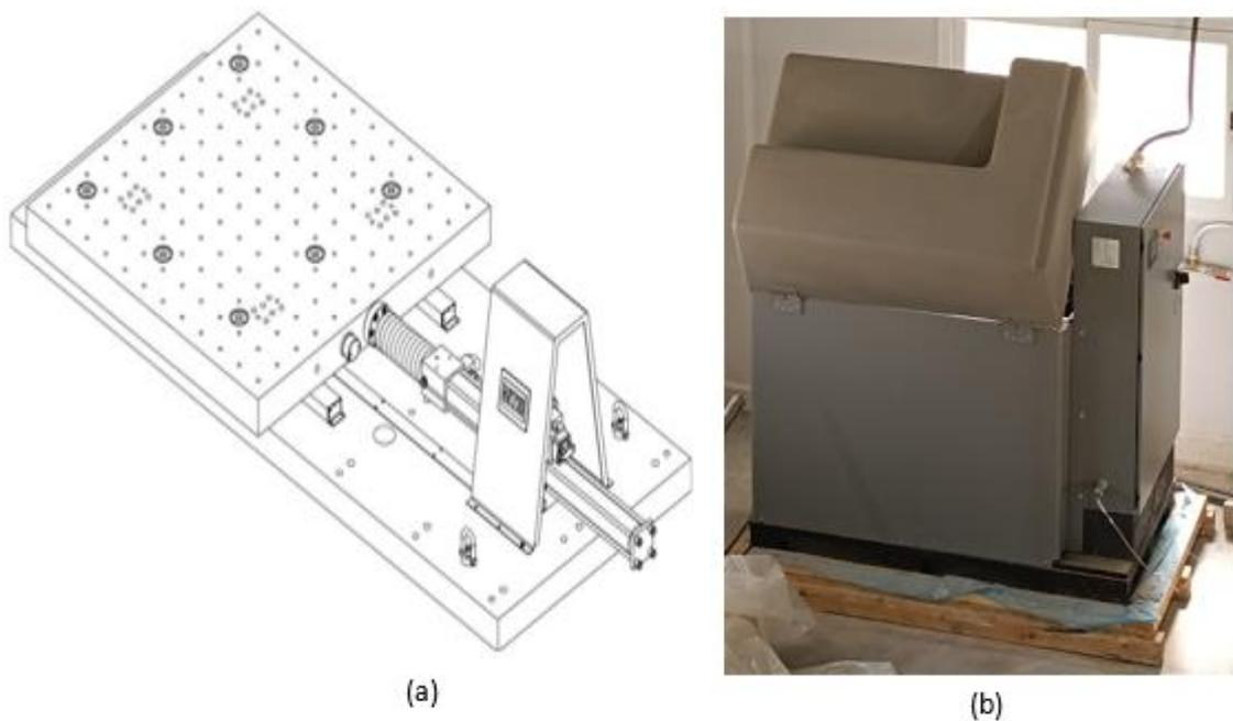
**Figure 1 – The main components of the shaking table of the RISAM laboratory**
