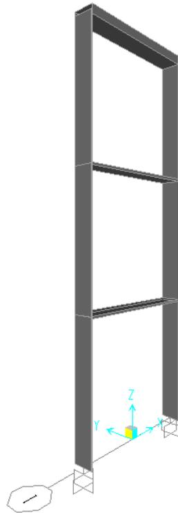
**Figure 7 – Three-dimensional finite elements model**
