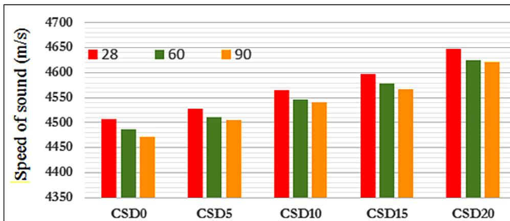
Figure 11 - Variation of the speed of sound function of type of concrete
