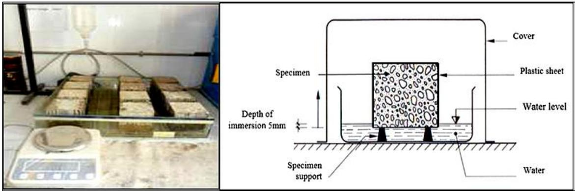
**Figure 5 - Diagram of the capillary water absorption test**
