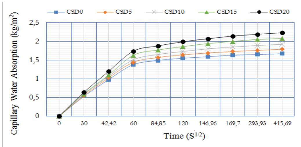
**Figure 7 - Water absorption by capillary action**
