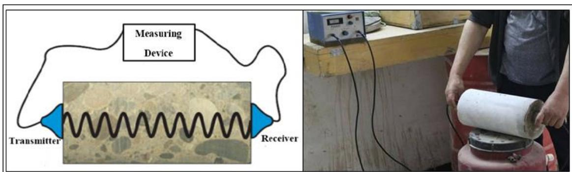
**Figure 9 - Measure the speed of sound**
