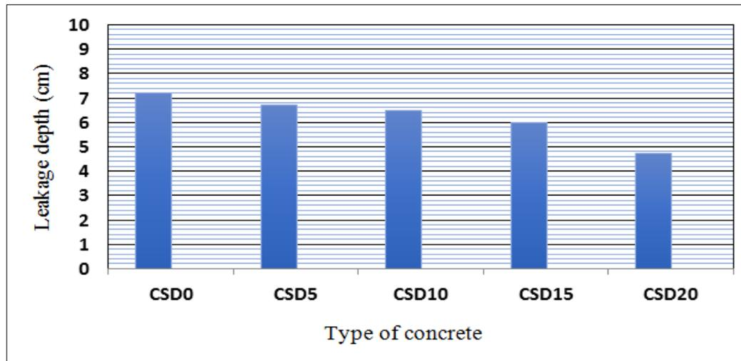
**Figure 3 - Results of Water Permeability for Various Concrete Types**
