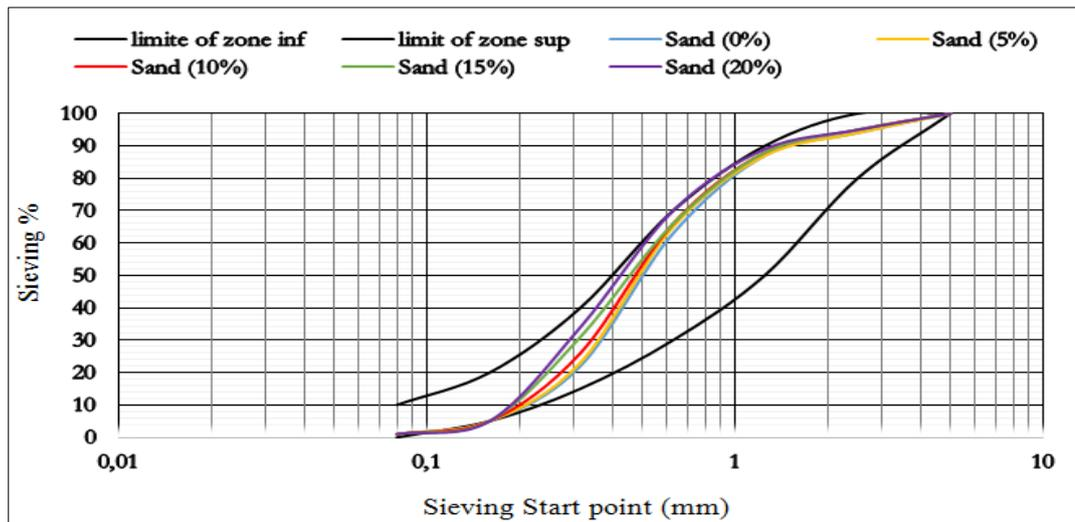
**Figure 1 - Grading Curves for Different Types of Sand**
