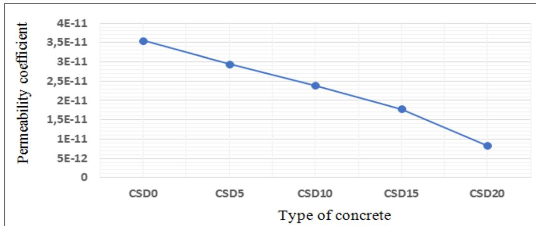
**Figure 4 - Permeability Coefficient Values for Each Type of Concrete**
