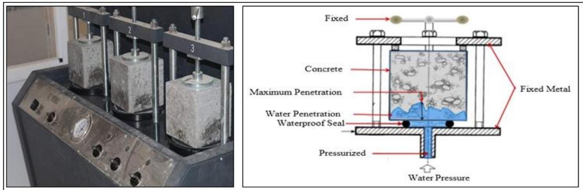
Figure 2 - Setup of the Sample in the Testing Apparatus
