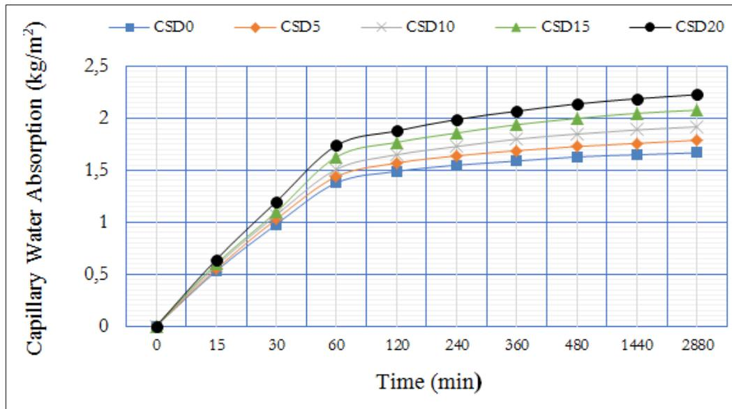
**Figure 6 - Water absorption by capillary action for different types of concrete**
