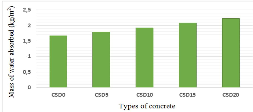
**Figure 8 - Water absorption by capillarity after 48 hours for different types of concrete**
