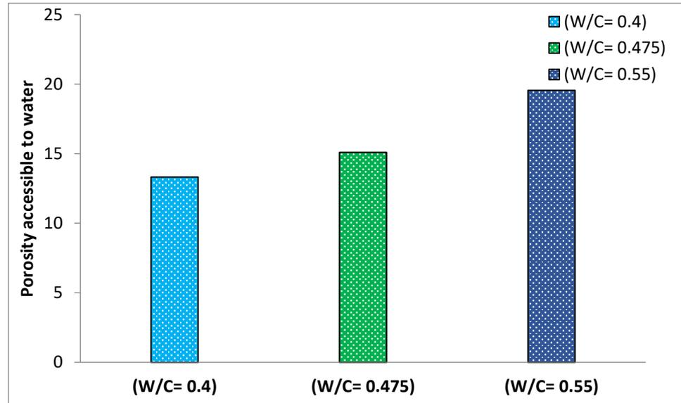
**Figure 6: Porosity Measurements of Self-Compacting Concrete at Various Water-to-Cement Ratios.**
