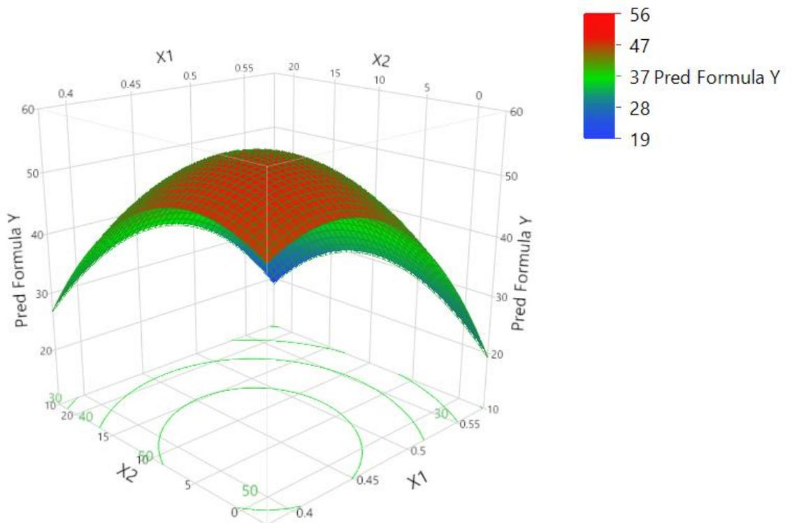
Figure 5 – Three-dimensional visualization of 28-day compressive strength variations based on water-cement ratio and powdered sand dose interactions using response surface analysis
