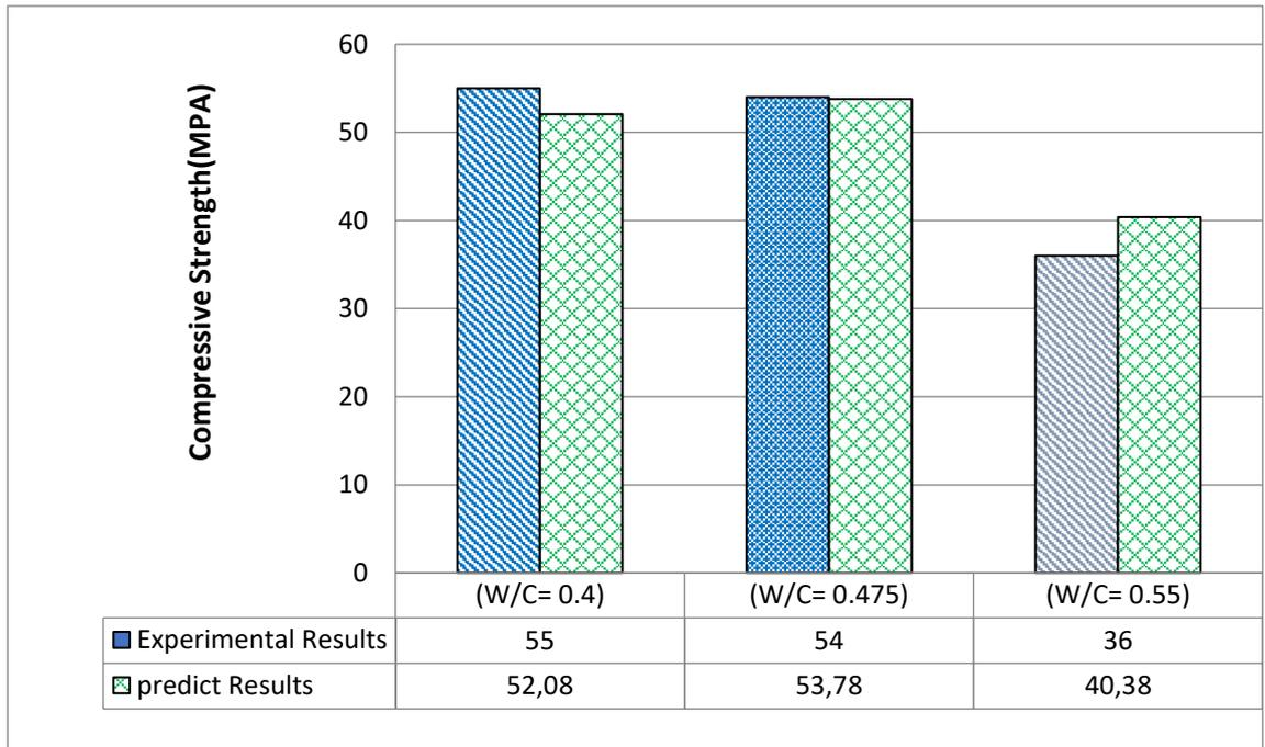
Figure 4 – Results of compressive strength at 28 days tests experimental and predict of E-SCC.
