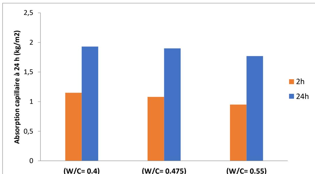
**Figure 7 – Effect of Water-Cement Ratio on Capillary absorption of E-SCC.**
