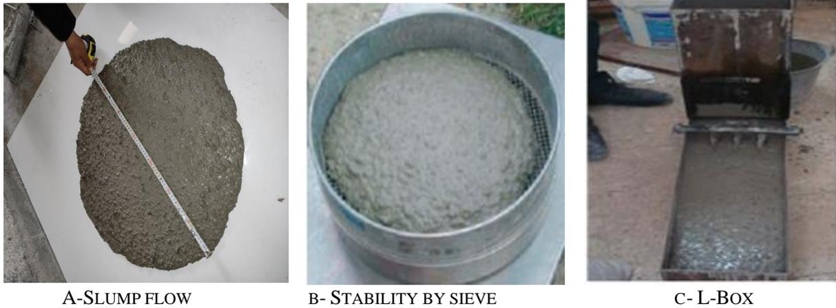
Figure 2 – Autoplacibility tests of E-SCC.
