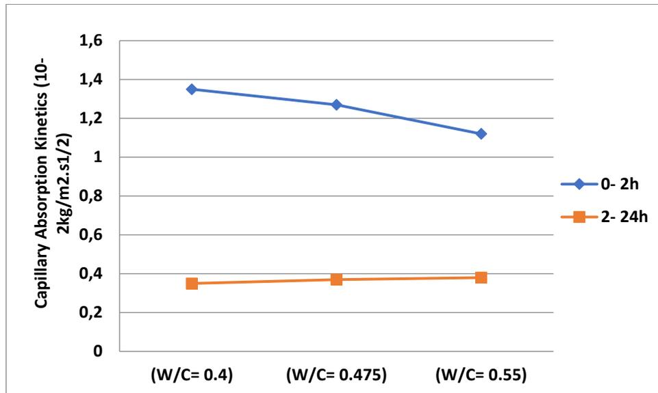
**Figure 8 – Effect of Water-Cement Ratio on Capillary absorption kinetics of E-SCC.**
