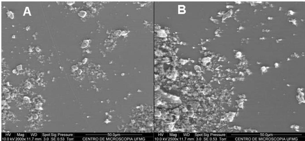
Figure 4 - Scanning electron micrographs of pure clay (A) and WTS (B).
