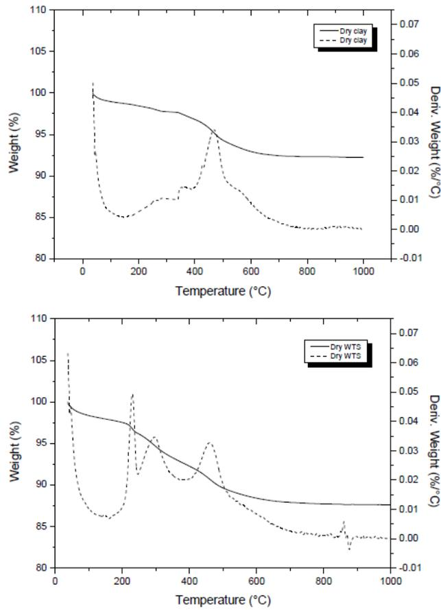
Figure 5 - TG/DTA thermograms of clay and WTS.
