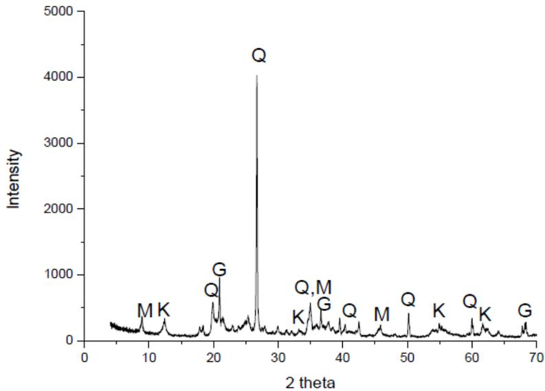
Figure 1 - X-ray diffraction patterns of WTS. Peaks are identified to following mineral phases: Q = quartz, K = kaolinite, G = gibbsite and M = muscovite.
