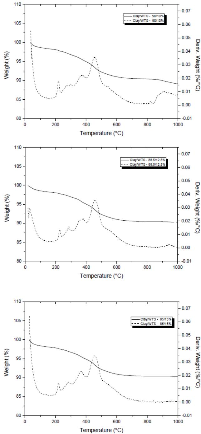
Figure 6 - TG/DTA thermograms of clay/WTS mixtures.
