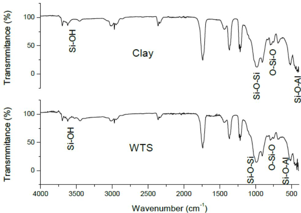
Figure 3 – FT-IR spectra of WTS and clay samples.
