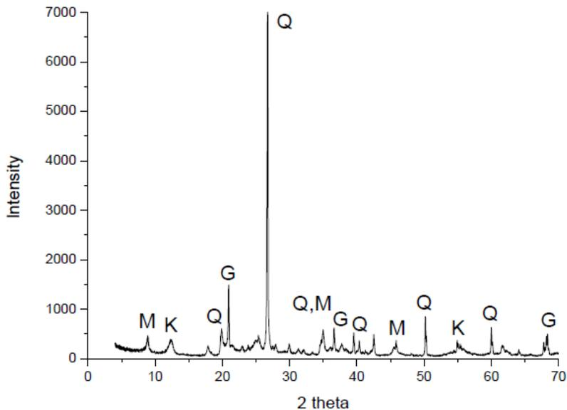
Figure 2 - X-ray diffraction patterns of clay. Peaks are identified to following mineral phases: Q = quartz, K = kaolinite, G = gibbsite and M = muscovite.
