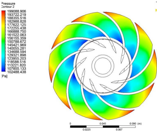
Figure 9 – Pressure distribution on ten blades rotor.
