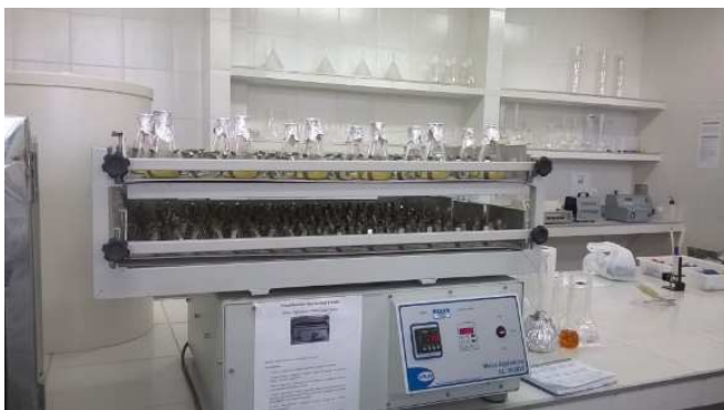
Figure 4 - Erlenmeyer flasks containing water, oil and biomass mixture under stirring on a vibratory table at 130 rpm.
