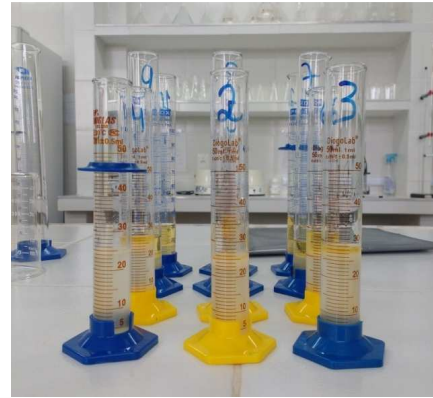
Figure 5 - Volumetric calibration of remaining gas volume in beakers.
