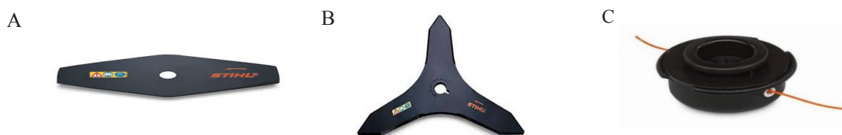
Figure 1. Cutting sets used in the brushcutter to carry out the experiment: double-ended blade (A); three-pronged blade (B); double nylon thread (C)
