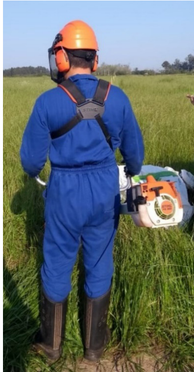
Figure 2. Operator with PPE, data collection sensors and side brushcutter
