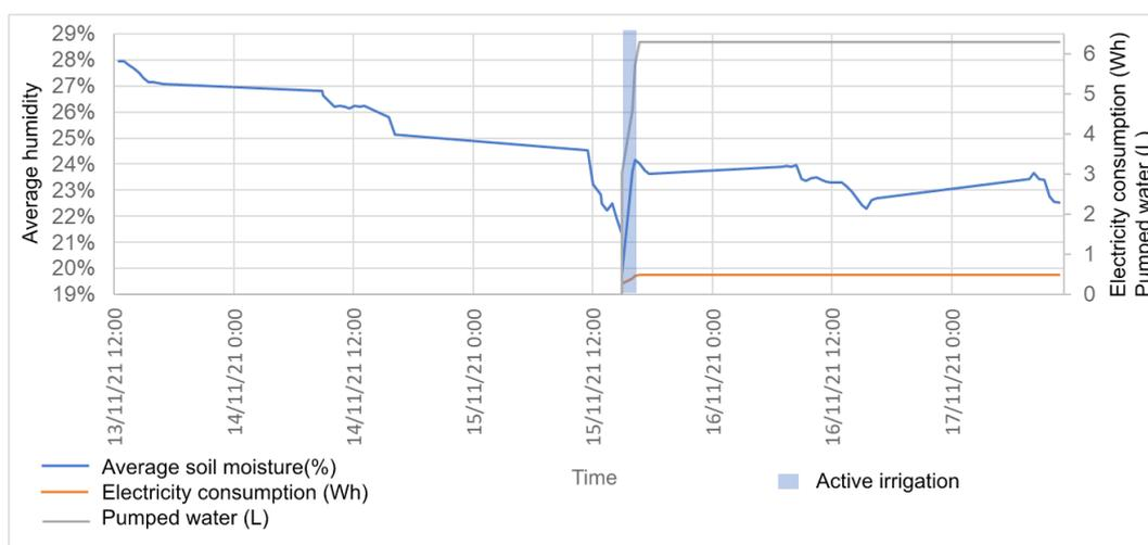
**Figure 11.** Irrigation test performed on substrate A
