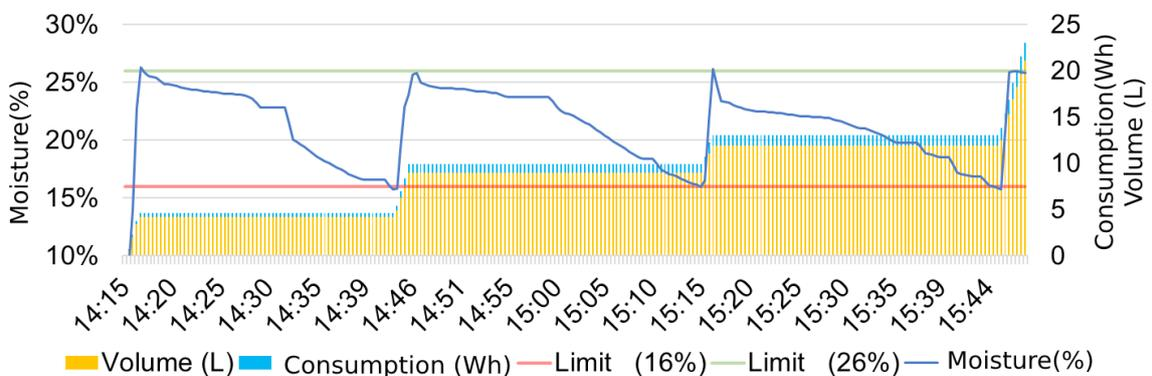
**Figure 14.** Irrigation test for substrate B and limits from 16 to 26%
