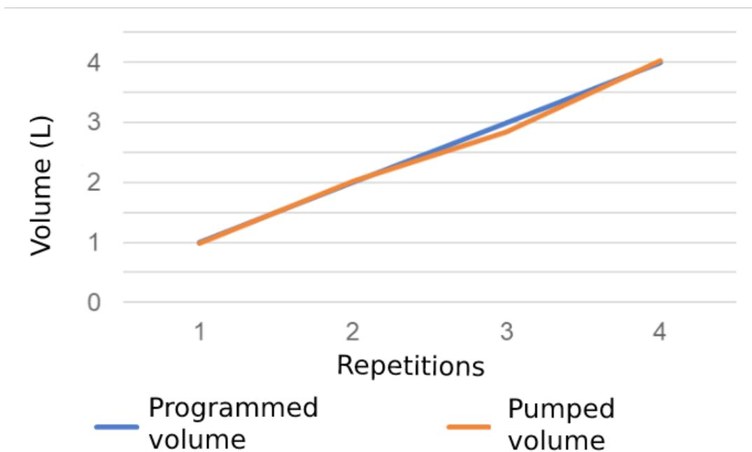
**Figure 10.** Result of the YF-S201 Flow Sensor Readings
