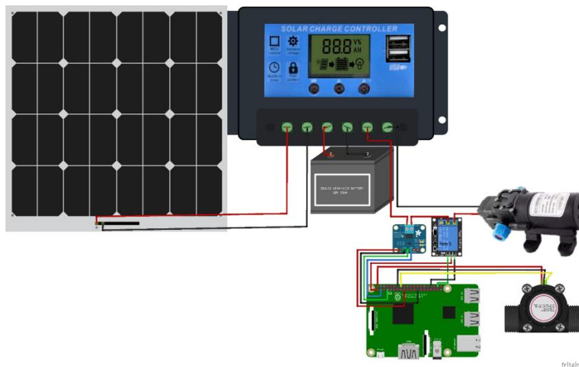
**Figure 4.** Wiring diagram of part 2 of the prototype
