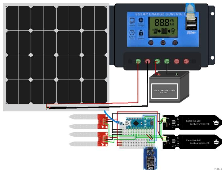
**Figure 3.** Wiring diagram of part 1 of the prototype
