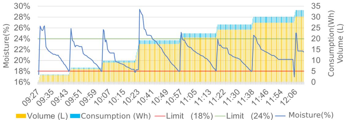
**Figure 13.** Irrigation test for substrate B and limits from 18 to 24%
