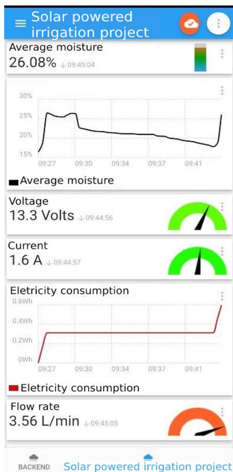
**Figure 16.** Screenshot of the IoT MQTT Panel application while the prototype is running at the time of irrigation on
