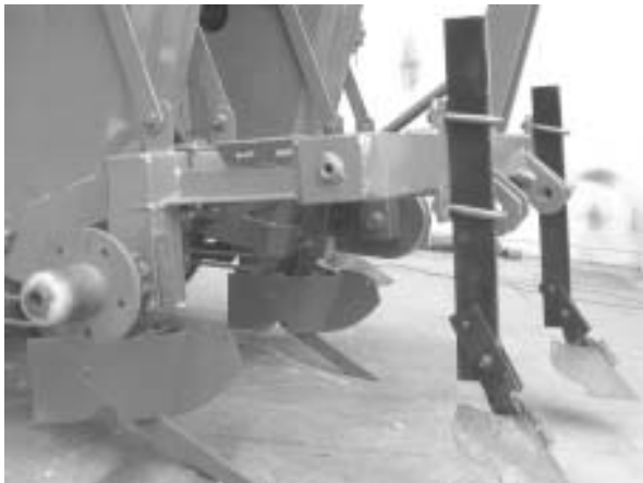
Figure 1. Side view of the mechanism adapted to the potato planting machine, showing the frontal furrower and the fertilizer separator with the plowing rod.
