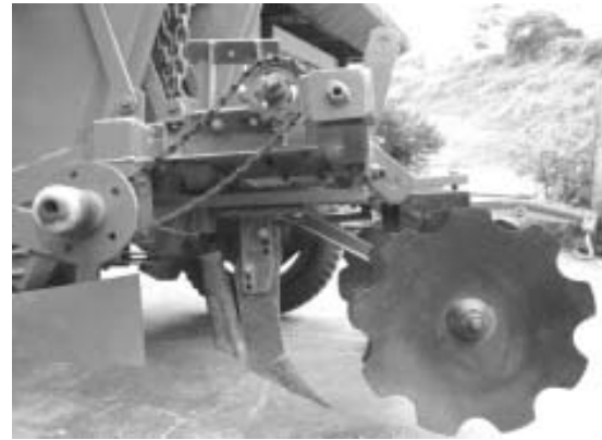
Figure 2. Side view of the mechanism adapted to the potato planting machine, showing the ensemble of disk harrows, boot-type furrower and fertilizer separator.
