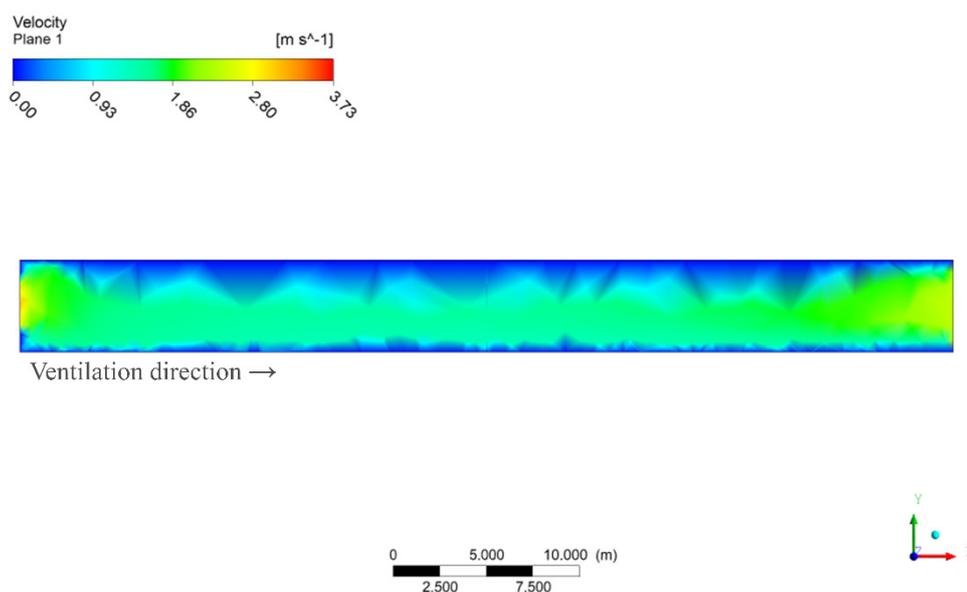
**Figure 3.** Air velocity plan along the barn length
