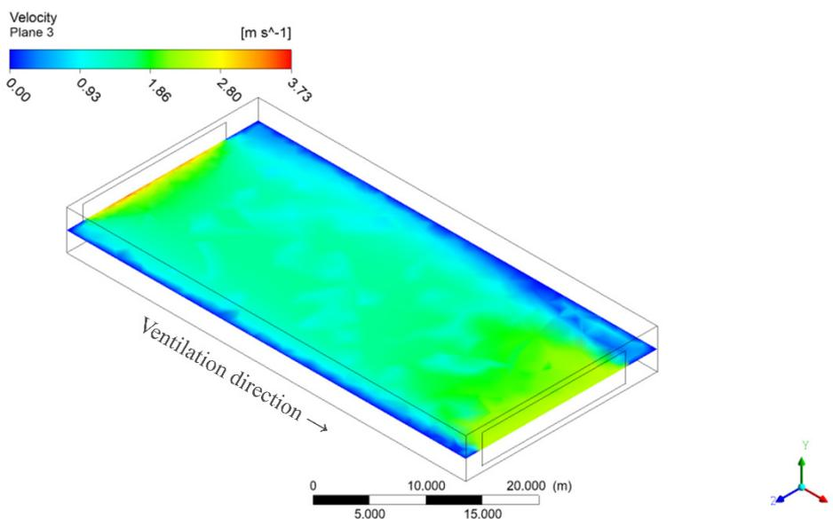
**Figure 2.** Air velocity plan inside the barn
