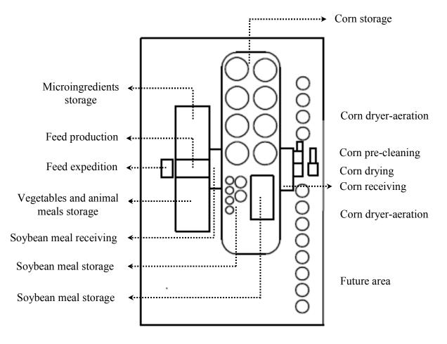
Figure 1. Partial feed milling plant and points of product loss sampling.
