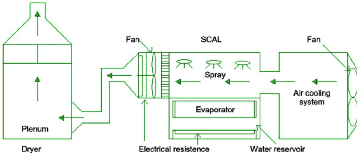
**Figure 1.** Drying system used for the mechanical drying of coffee. Source: Adapted from Alves (2013)
