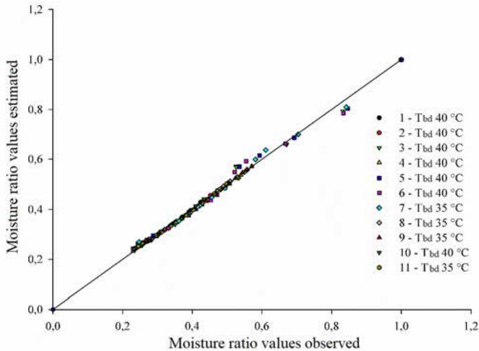
**Figure 2.** Moisture ratio values (dimensionless) observed (x-axis) and estimated (y-axis) by the Diffusion Approximation model for the first part of the drying of coffee grains
