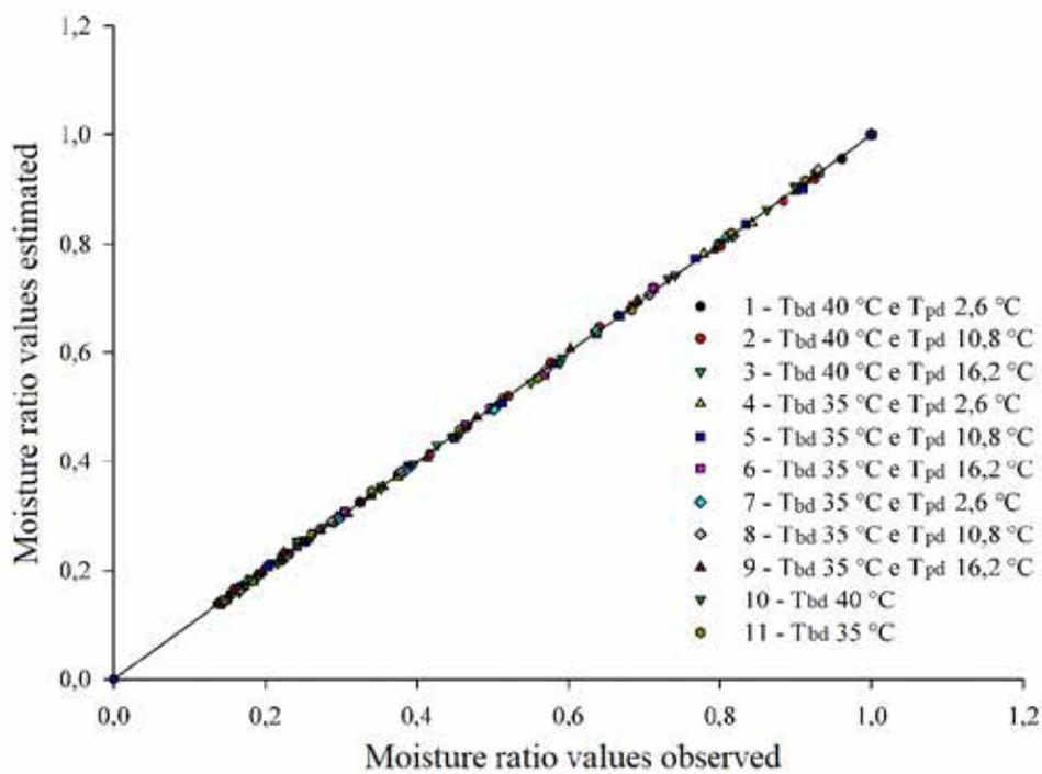
**Figure 3.** Moisture ratio values (dimensionless) observed (x-axis) and estimated (y-axis) by the Modified Midilli model for drying coffee grains after partial drying (second part of drying)
