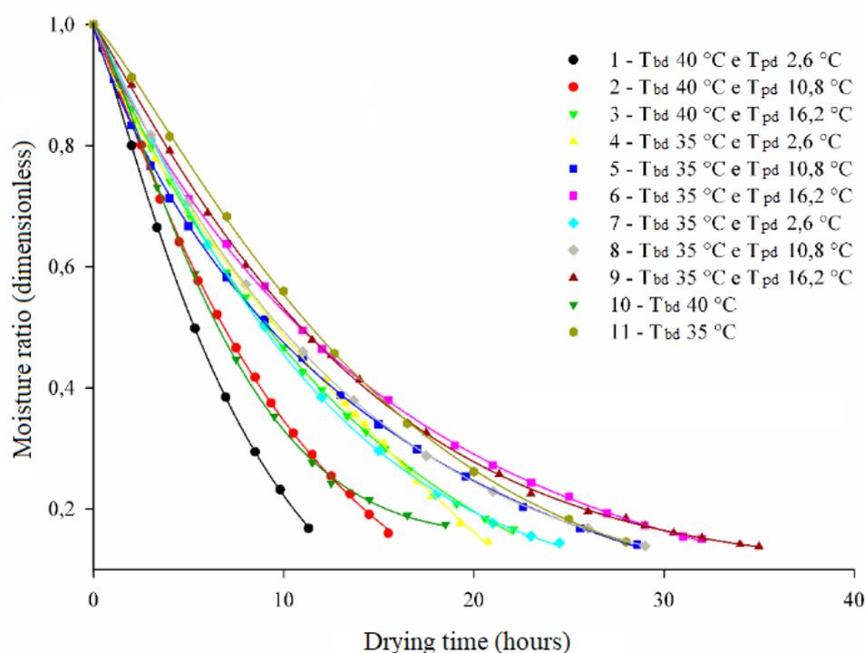
**Figure 5.** Moisture ratio values observed and estimated (y-axis) by the Modified Midilli model for the second part of the drying of the peeled coffee, as a function of the drying time (x-axis)
