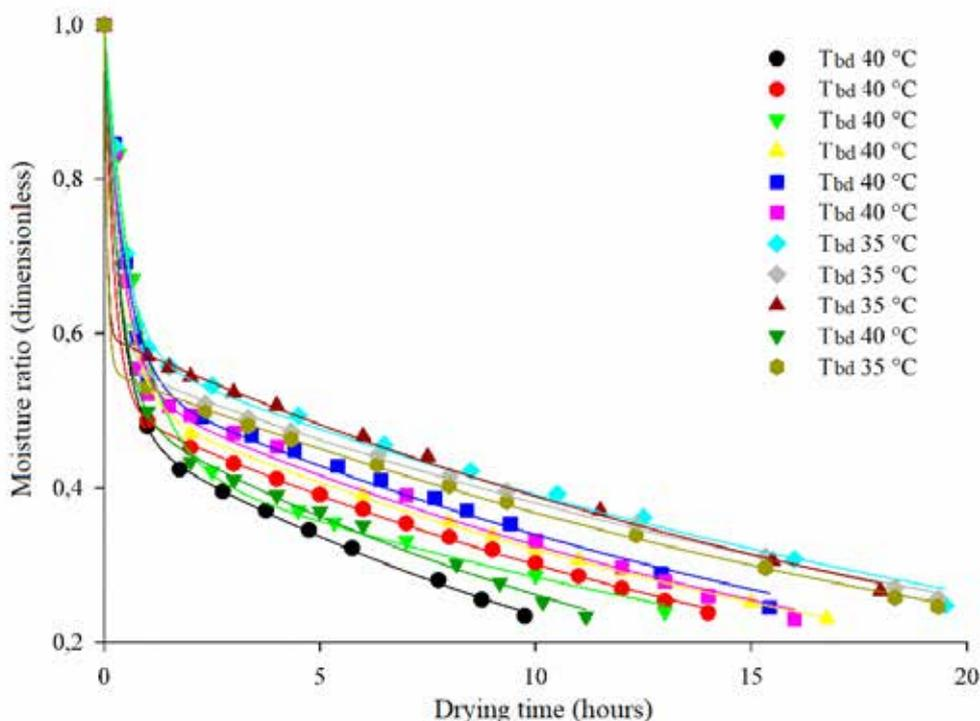
**Figure 4.** Moisture ratio values observed and estimated (y-axis) by the Diffusion Approximation model for the first part of the drying of the peeled coffee, as a function of the drying time (x-axis)
